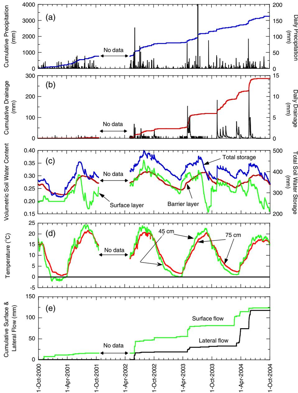
**Fig. 4.** (a) Precipitation, (b) drainage, (c) volumetric soil water content, (d) soil temperature, and (e) surface and lateral flow data from the test section at Cedar Rapids, IA. The indicated depths of the temperature data are the bottom of the surface soil layer (45 cm) and the top of the soil barrier layer (75 cm).
