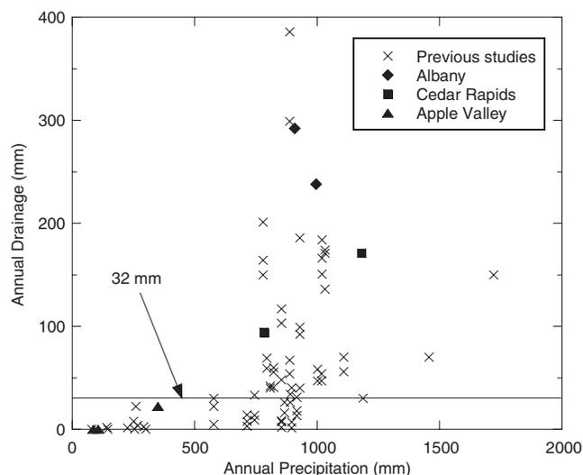
**Fig. 8. Annual drainage as a function of annual precipitation for the three sites in this study as well as past studies described in the literature. The annual drainage from a soil with saturated hydraulic conductivity ( $K_s = 1 \times 10^{-7} \text{ cm s}^{-1}$  at saturation and unit gradient conditions is 32 mm.**
