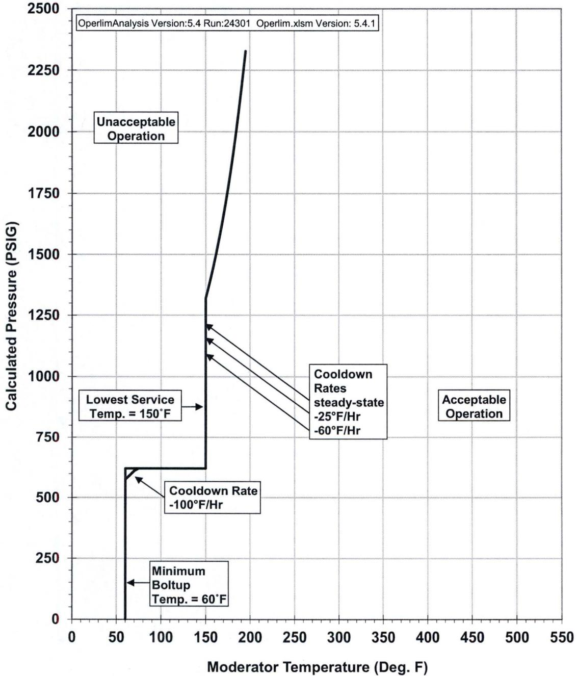
**Figure 8-2 Arkansas Nuclear One Unit 2 Reactor Coolant System Cooldown Limitations (Cooldown Rates of 0, 25, 60, and 100°F/hr) Applicable for 54 EFPY (with Flange and LST Requirements and without Margins for Instrumentation Errors) using the 1998 through the 2000 Addenda App. G Methodology (w/ K<sub>IC</sub>)**
