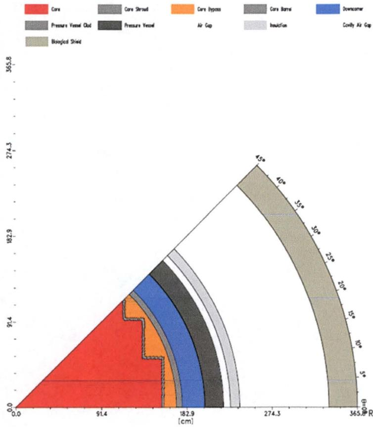
**Figure 2-2** Arkansas Nuclear One Unit 2 r,θ Reactor Geometry Plan View at the Core Midplane without Surveillance Capsules
