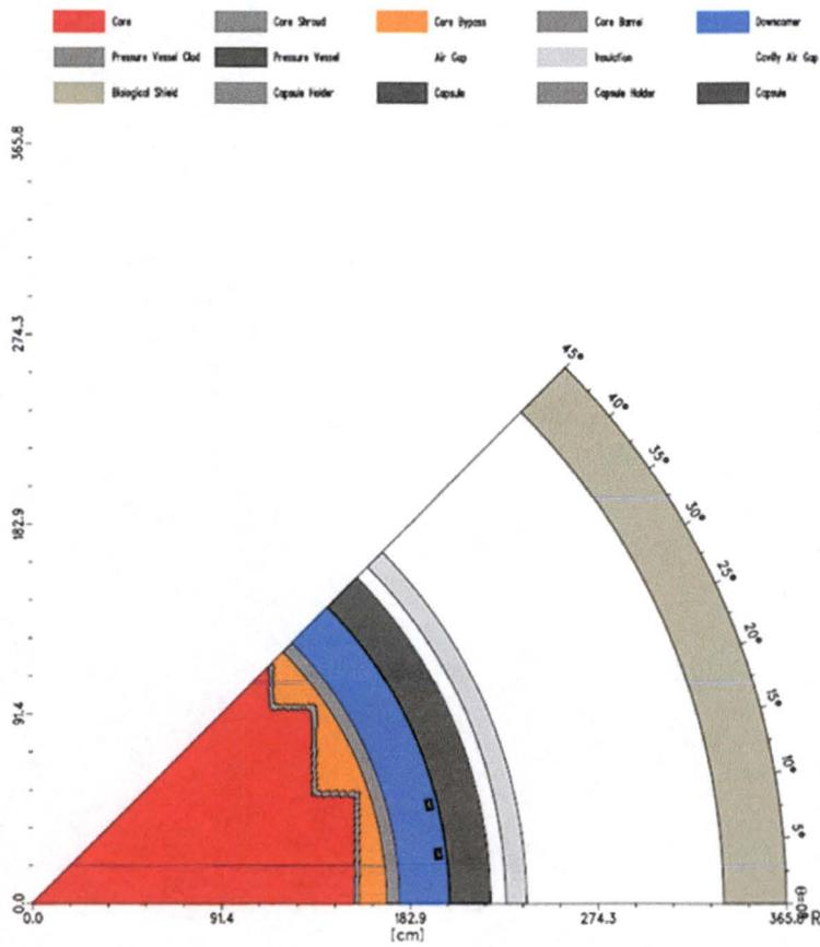
Figure 2-1 Arkansas Nuclear One Unit 2 r,θ Reactor Geometry Plan View at the Core Midplane with Surveillance Capsules
