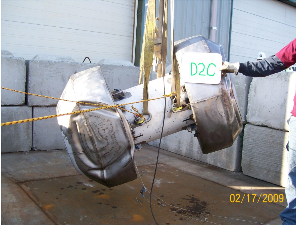
Figure 2.12.3-36 - Free Drop Test D2C Orientation
