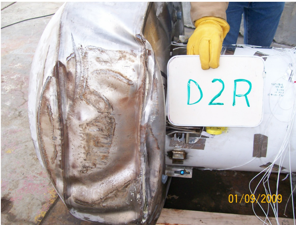
Figure 2.12.3-22 - Free Drop Test D2R, View of Torn Corner Joint
