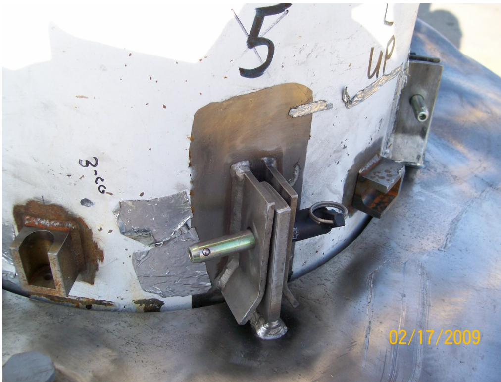
Figure 2.12.3-37 - Attachment Location #5 After Free Drop D2C
