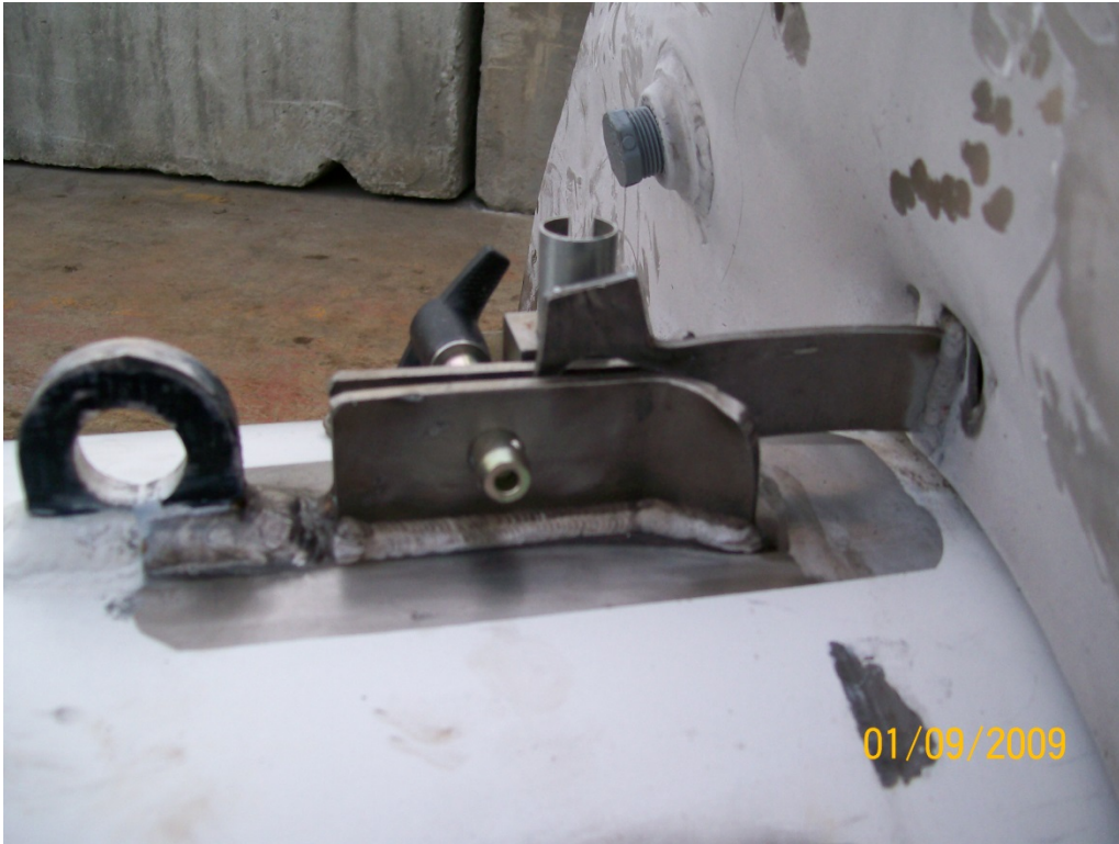
Figure 2.12.3-21 - Free Drop Test D2R, Close-up View of Failed Attachments
