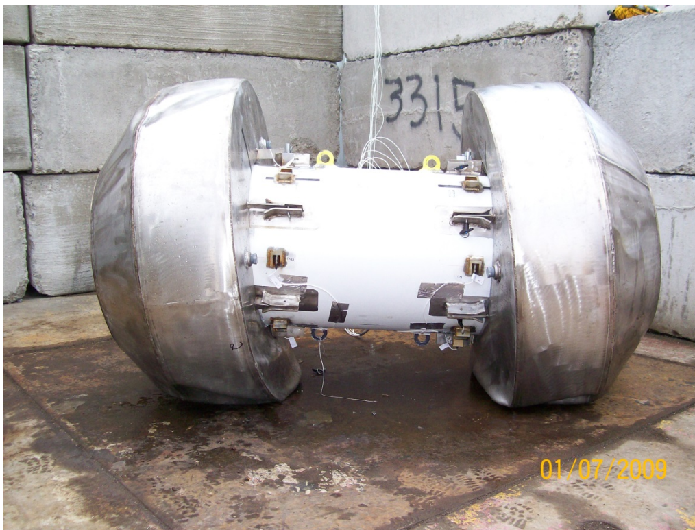
Figure 2.12.3-14 - Free Drop Test D2 Post-test Configuration
