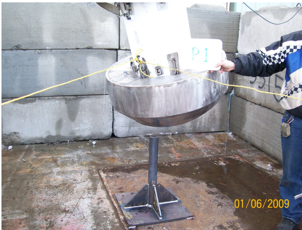
Figure 2.12.3-10 - Puncture Test P1 Orientation
