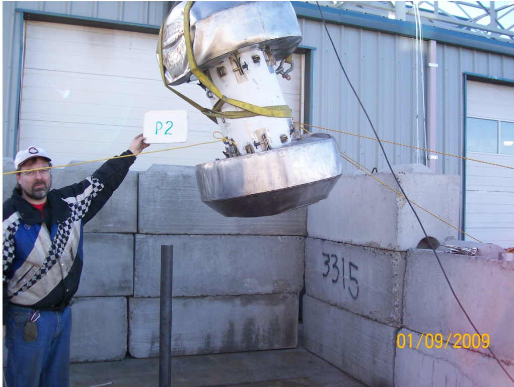
Figure 2.12.3-23 - Puncture Test P2 Orientation
