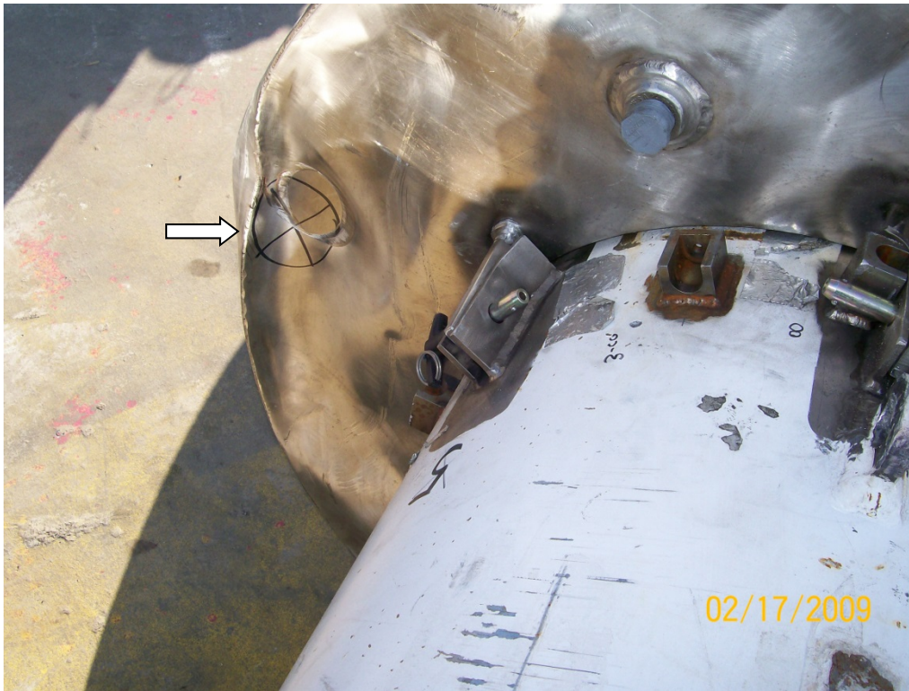
Figure 2.12.3-40 - Puncture Test P2C Result
