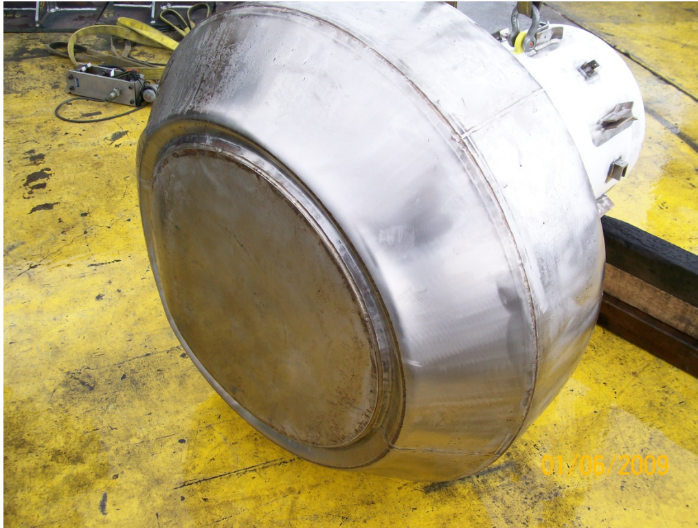
Figure 2.12.3-9 - Free Drop Test D1 Outside-In Deformation
