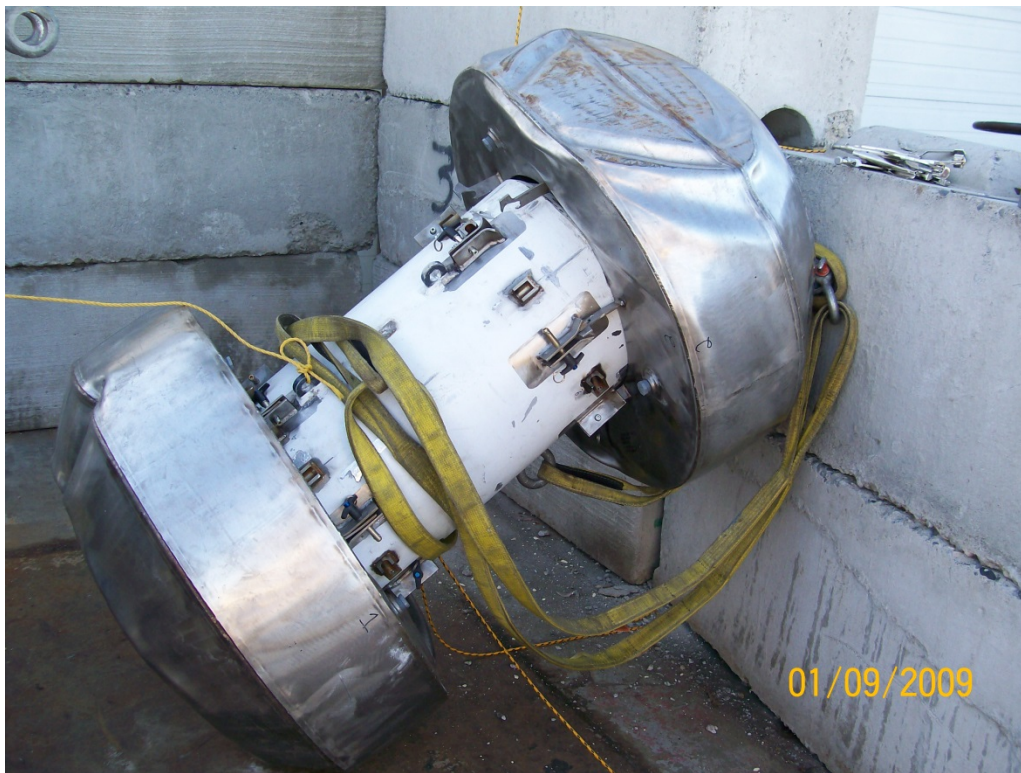
Figure 2.12.3-24 - Puncture Test P2 Result
