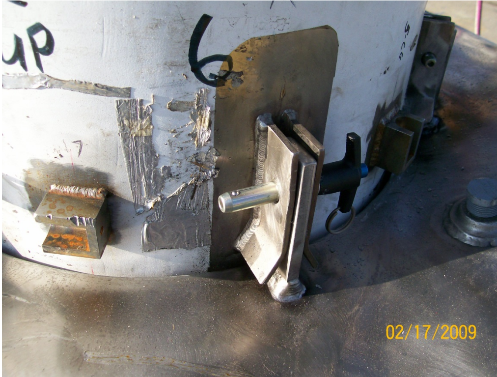
Figure 2.12.3-38 - Attachment Location #6 After Free Drop D2C
