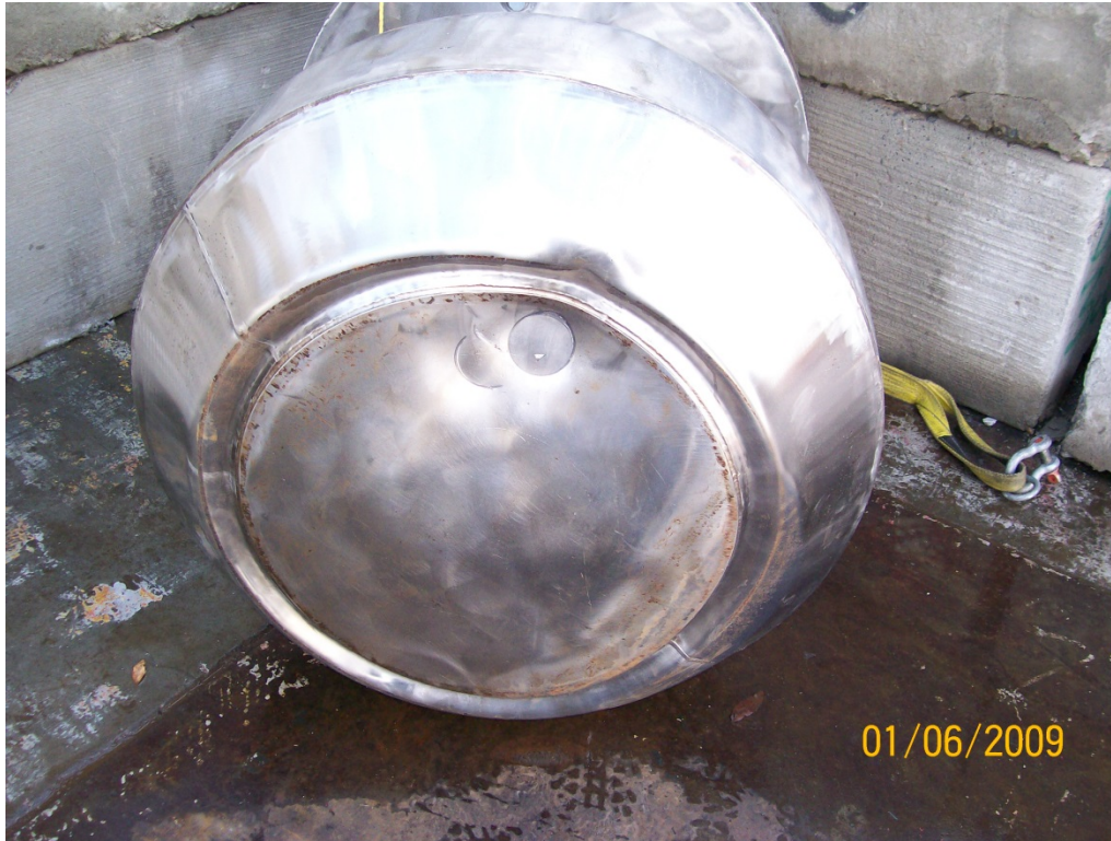
Figure 2.12.3-11 - Puncture Test P1 Deformation
