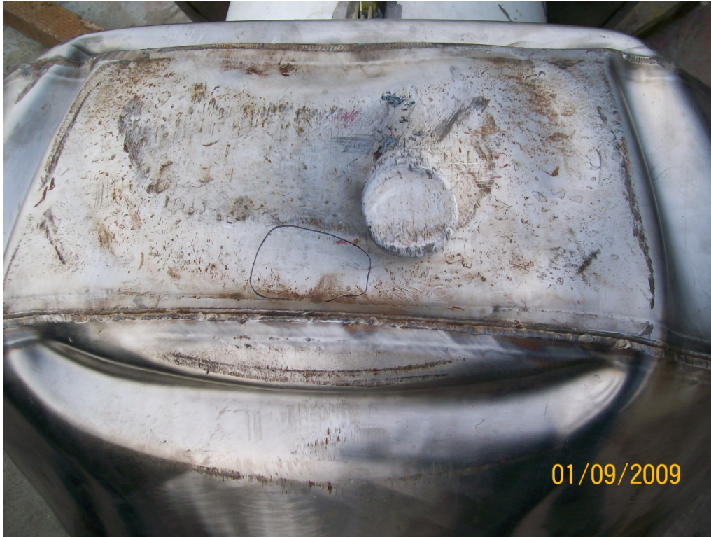
Figure 2.12.3-34 - Puncture Test P3 Damage
