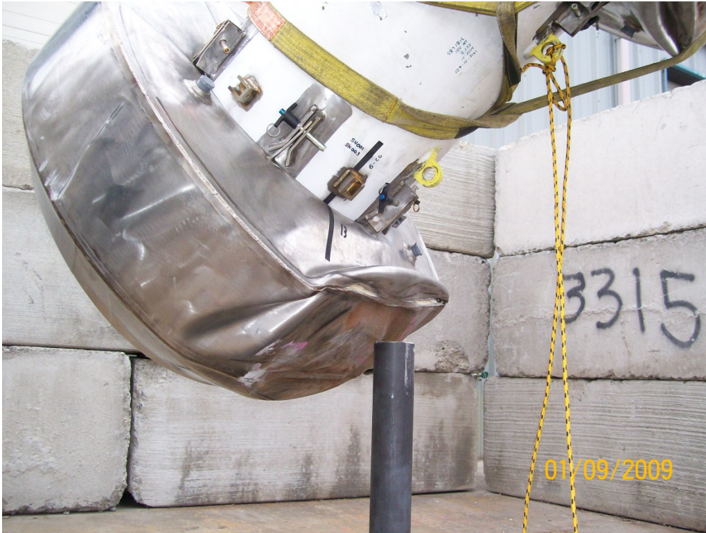
Figure 2.12.3-30 - Puncture Test P5 Orientation
