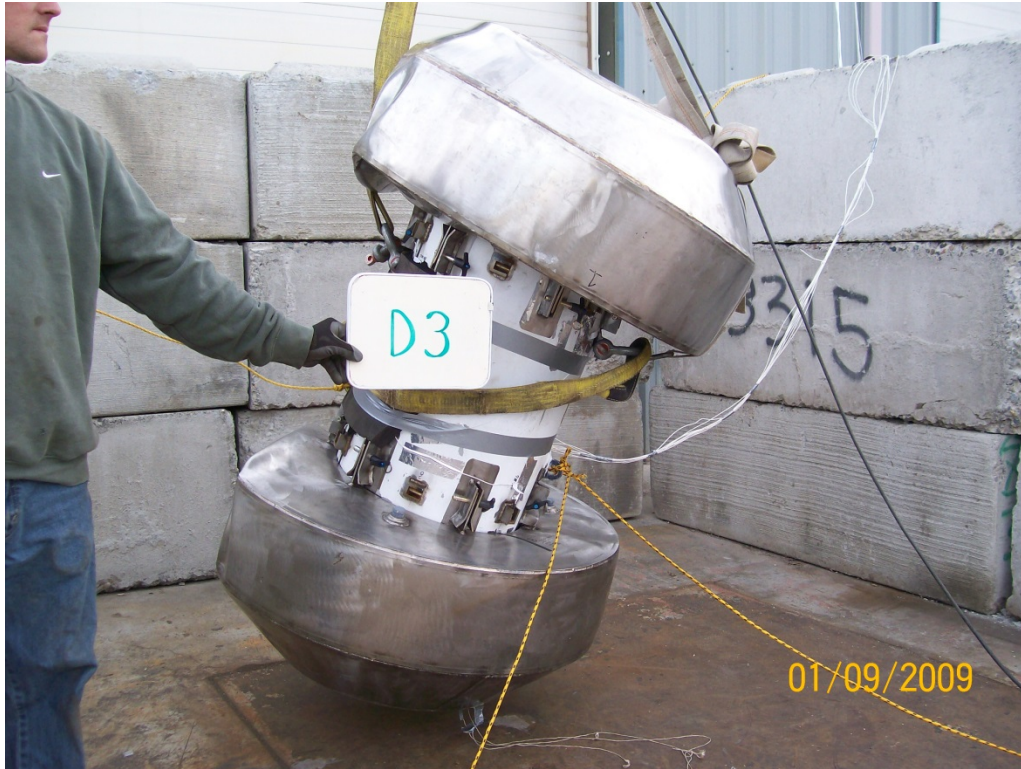
Figure 2.12.3-25 - Free Drop Test D3 Orientation
