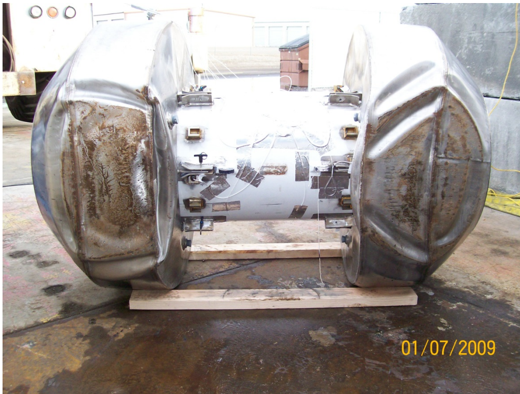
Figure 2.12.3-17 - Free Drop Test D2 Impact Deformation Surfaces
