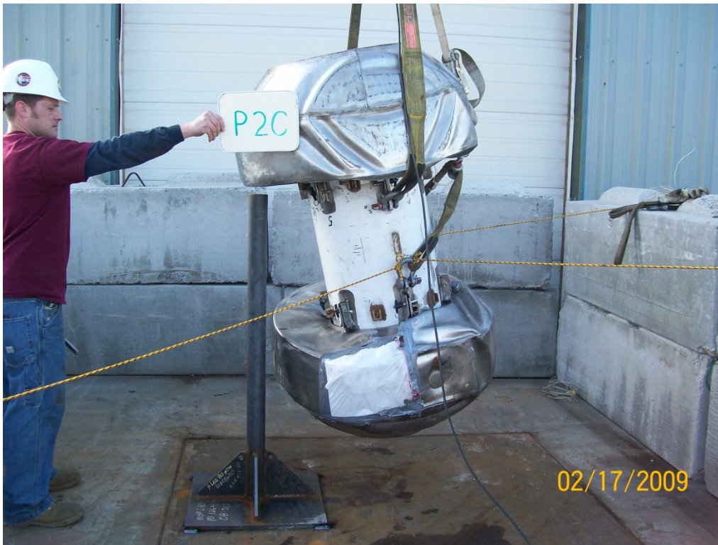
Figure 2.12.3-39 - Puncture Test P2C Orientation
