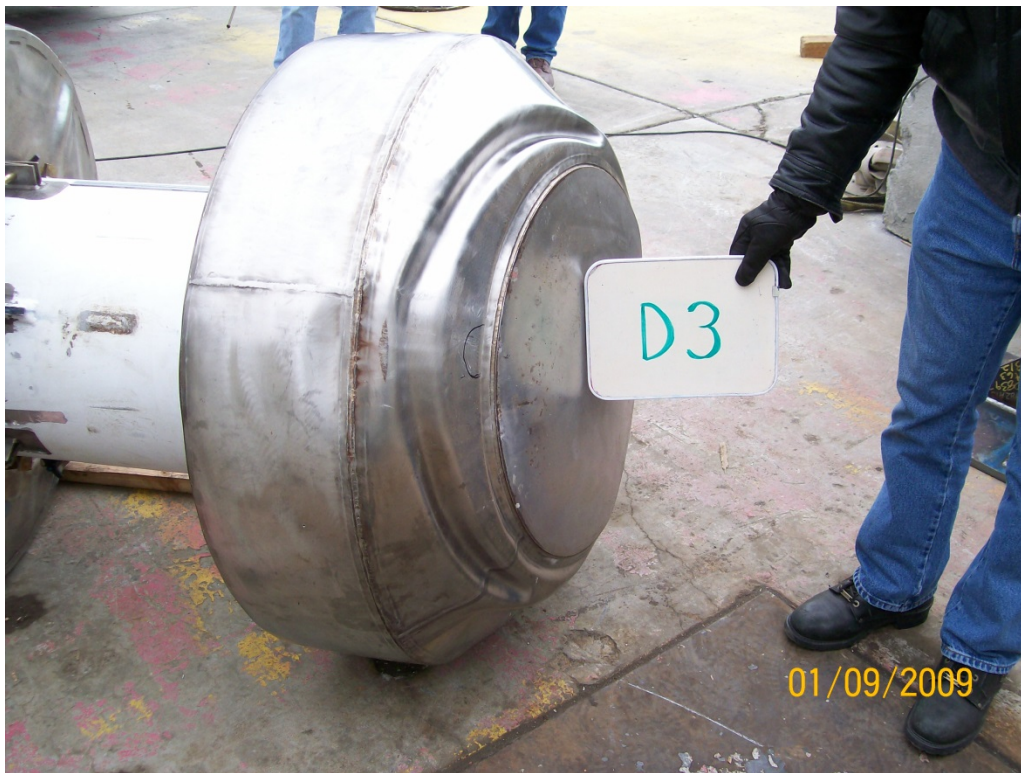
Figure 2.12.3-26 - Free Drop Test D3 Deformation
