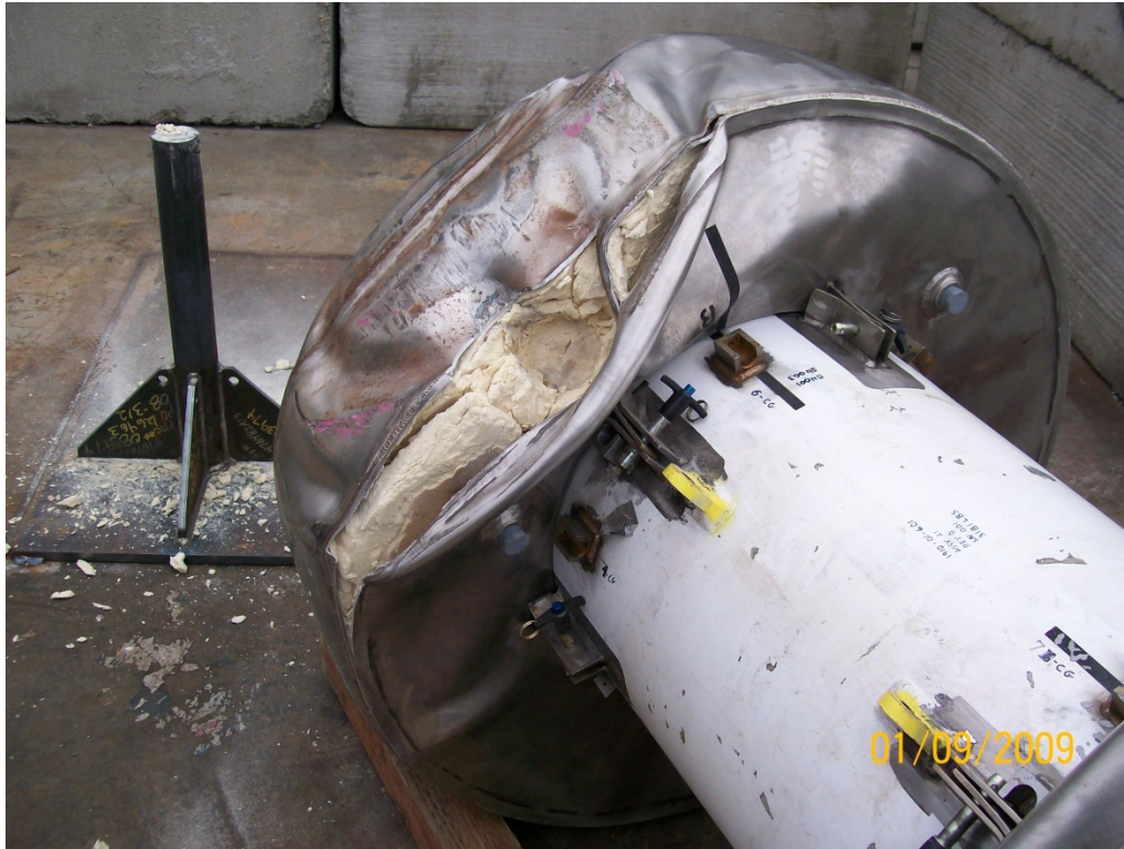
Figure 2.12.3-32 - Puncture Test P5 Damage
