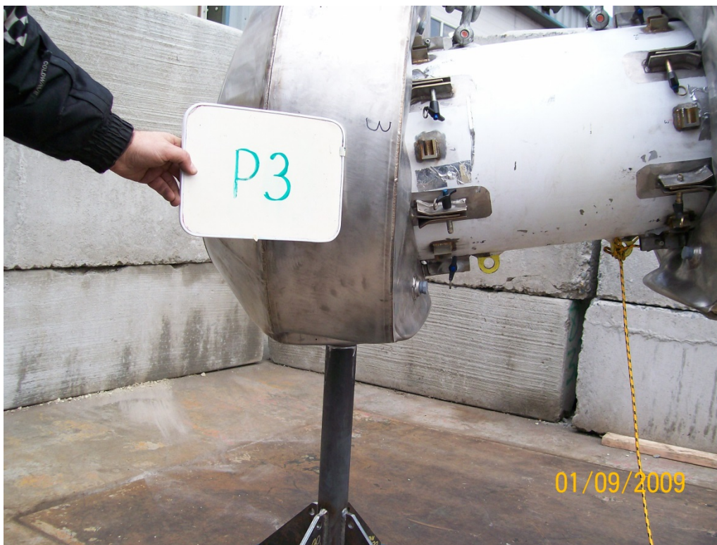
Figure 2.12.3-33 - Puncture Test P3 Orientation
