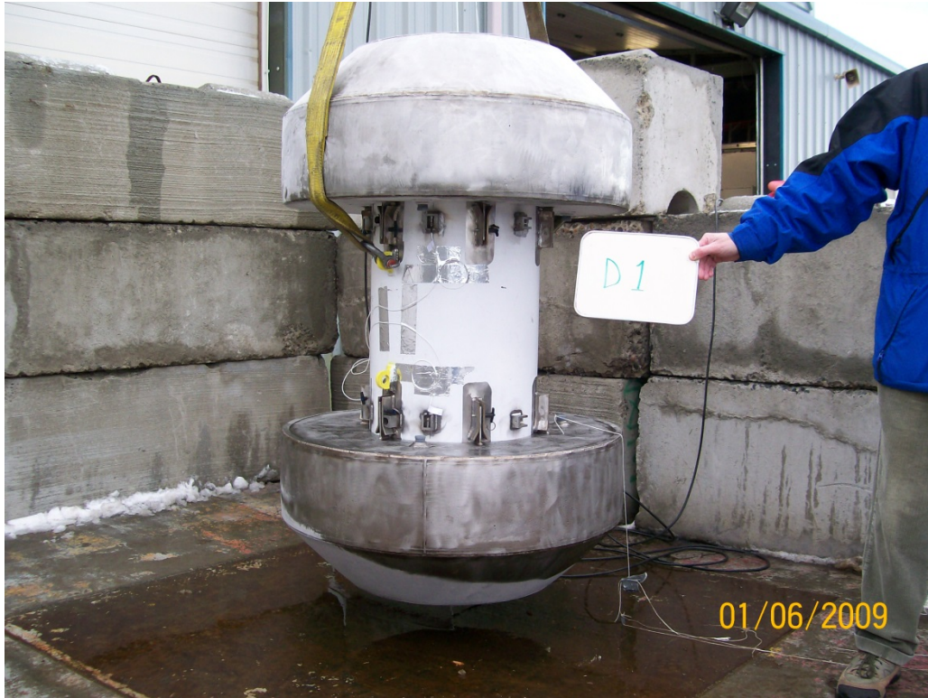
Figure 2.12.3-7 - Free Drop Test D1 Orientation
