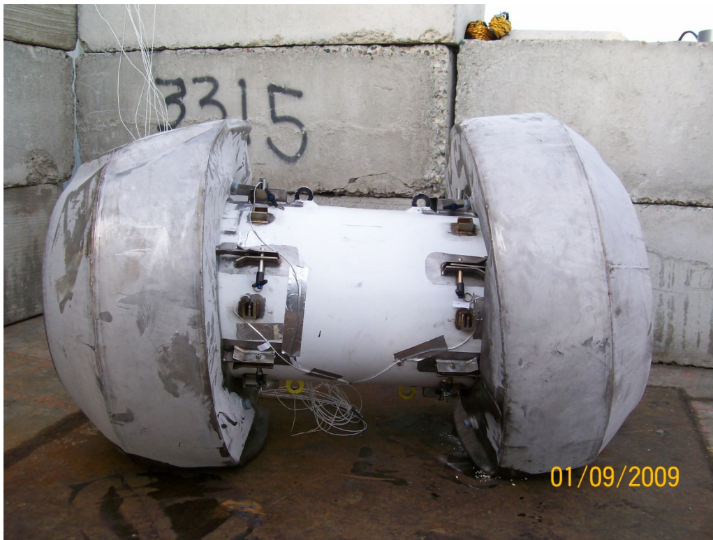
Figure 2.12.3-19 - Free Drop Test D2R Post-test Configuration
