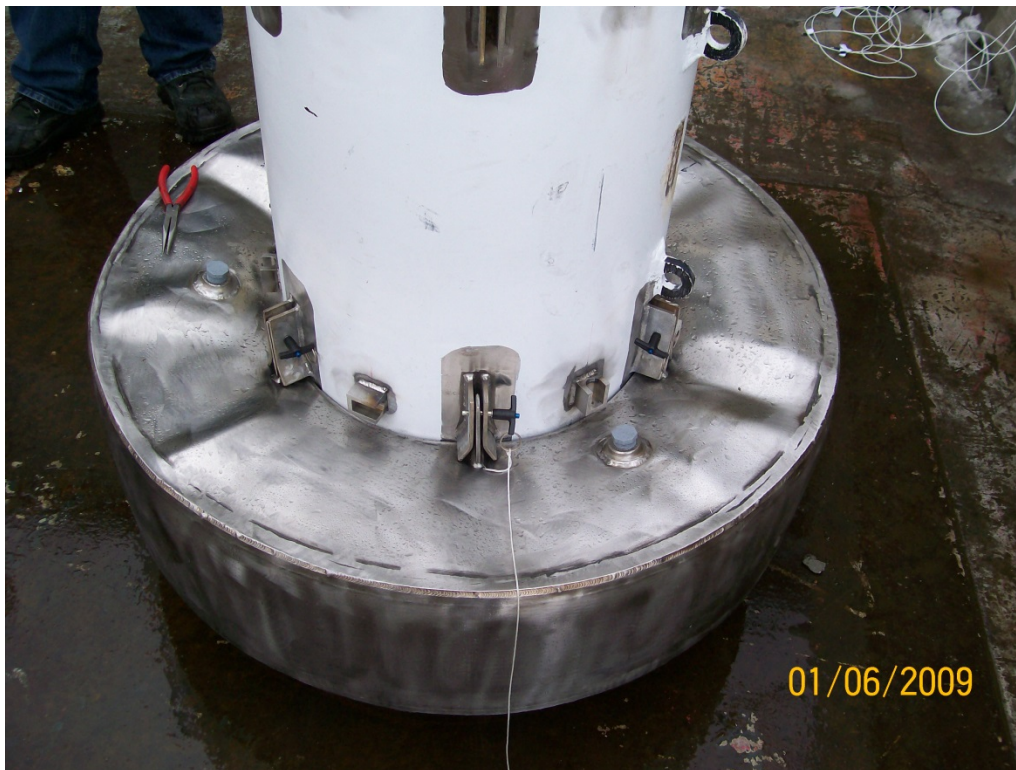
Figure 2.12.3-8 - Free Drop Test D1 Inside-Out Deformation
