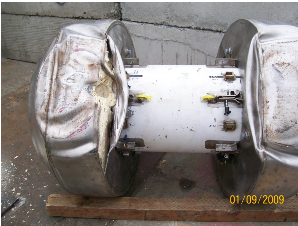
Figure 2.12.3-31 - Puncture Test P5 Damage
