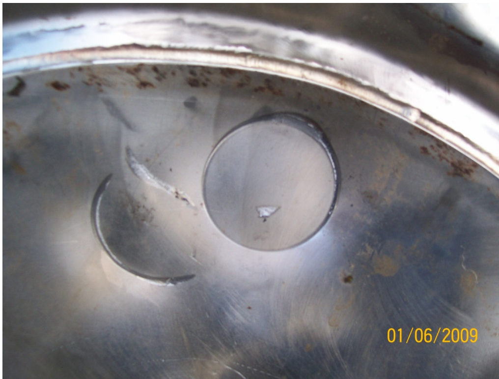
Figure 2.12.3-12 - Puncture Test P1 Deformation – Close-up View
