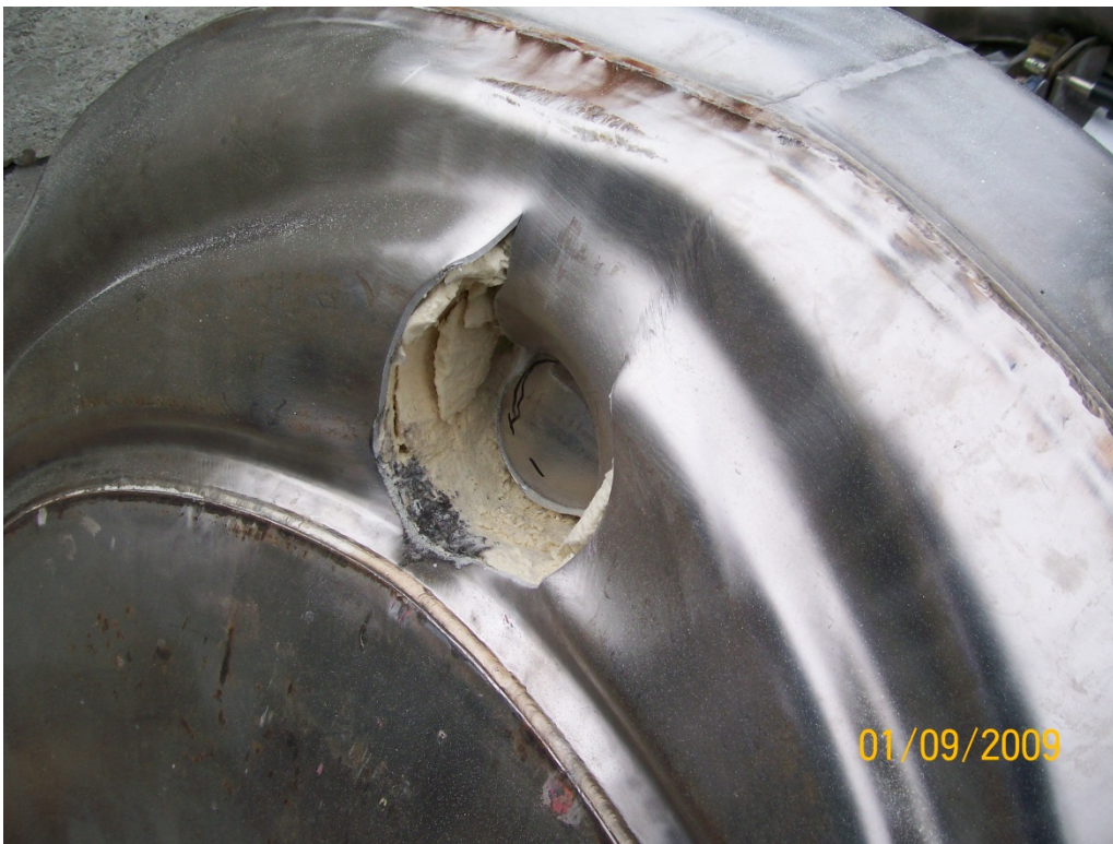
Figure 2.12.3-29 - Puncture Test P4 Damage
