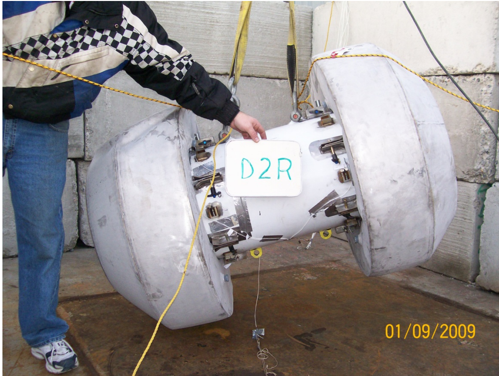
Figure 2.12.3-18 - Free Drop Test D2R Orientation
