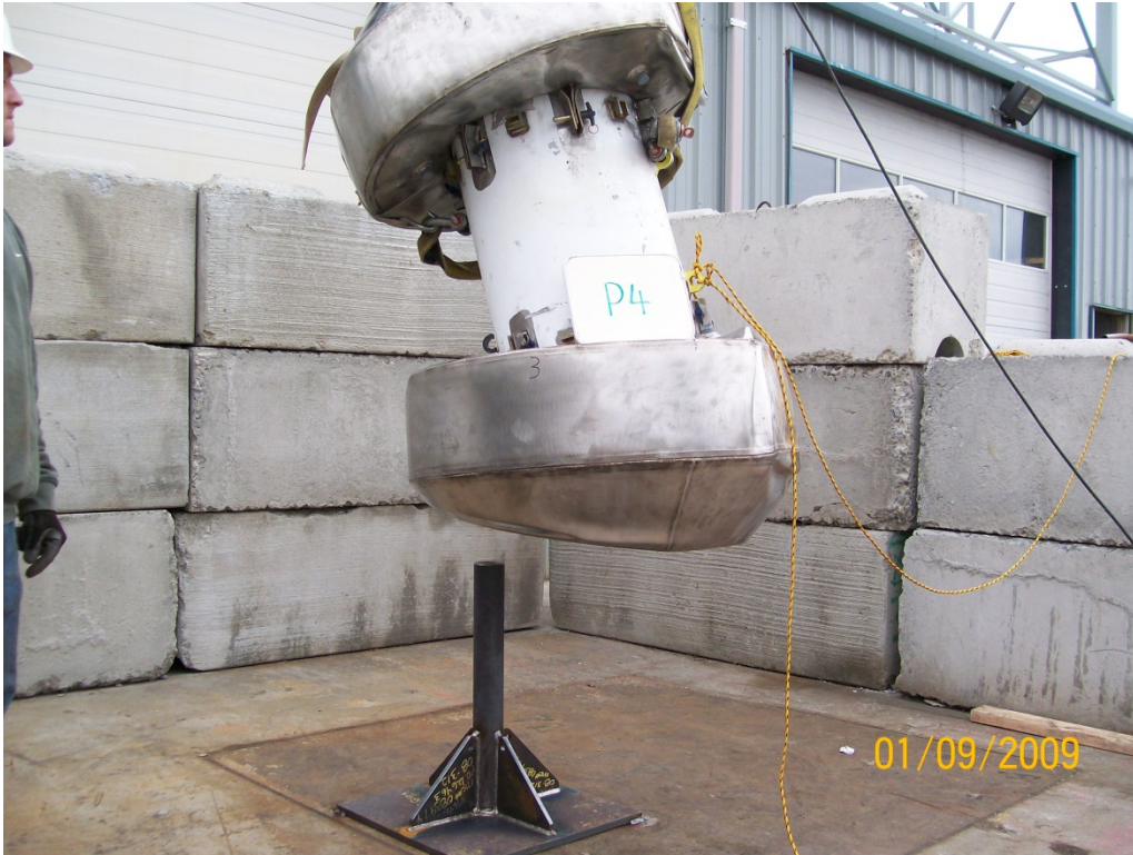
Figure 2.12.3-28 - Puncture Test P4 Orientation
