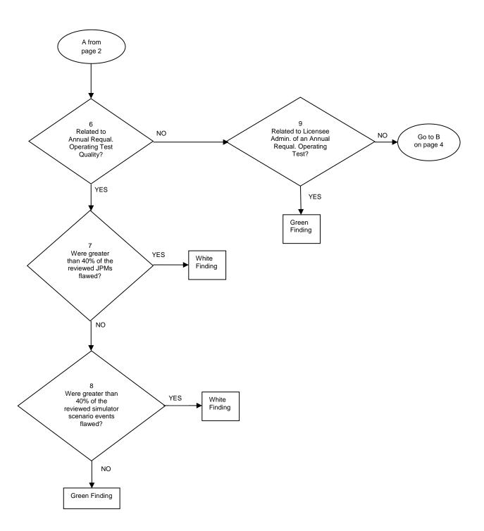
Figure I.1 – Licensed Operator Requalification SDP Flowchart (continued)
