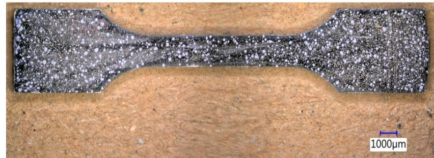
Placement of individual irradiated miniature tensile specimen onto small raised platform and example of good speckle pattern
