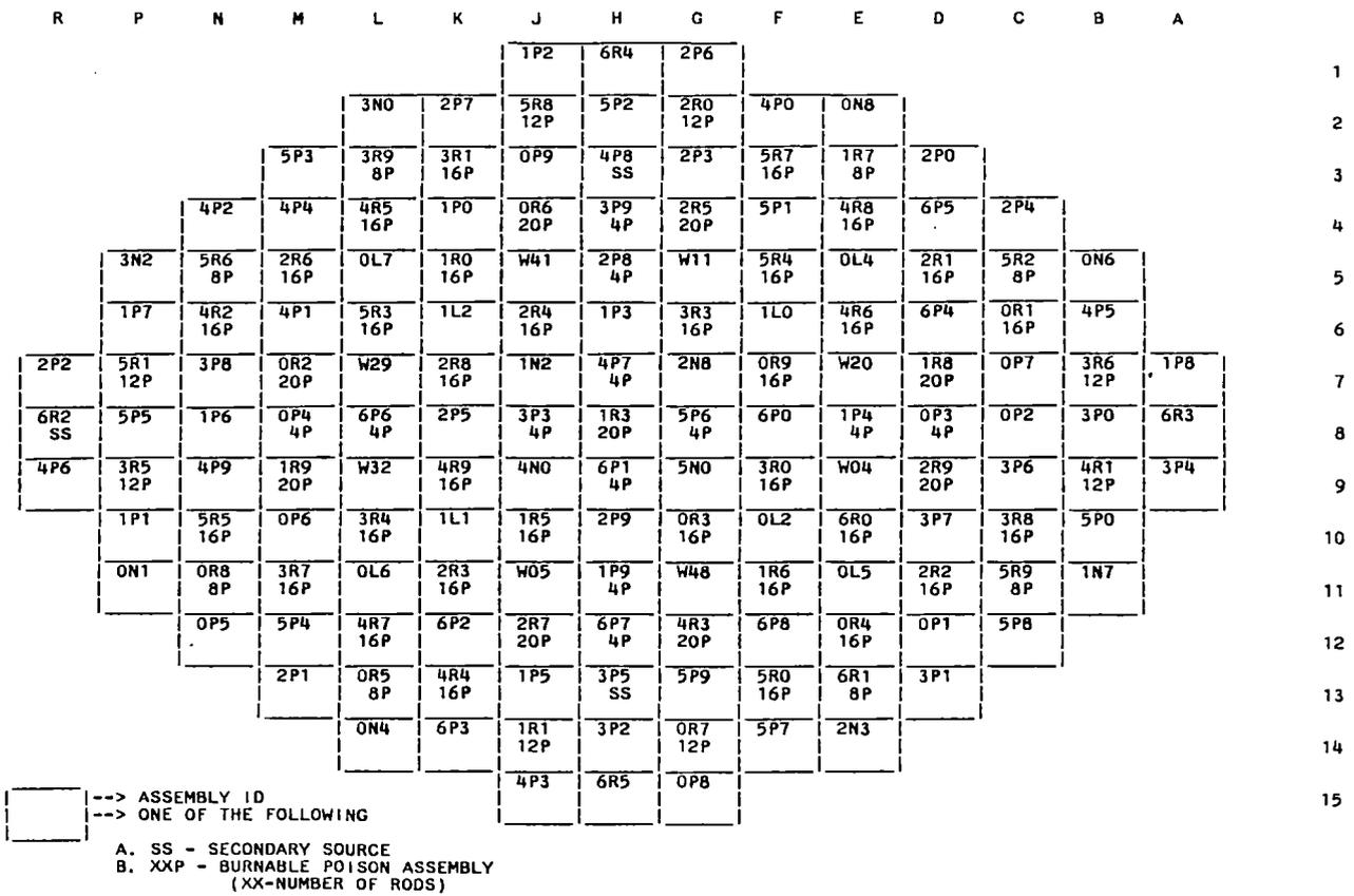
FUEL ASSEMBLY DESIGN PARAMETERS
