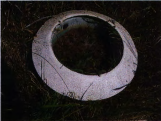
Figure 4-4: Lysimeter with Weather Protective Sleeve
