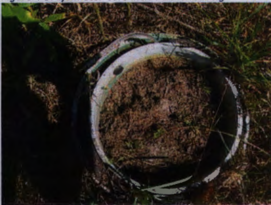
Figure 4-3: Lysimeter Core Inside Outer Casing
