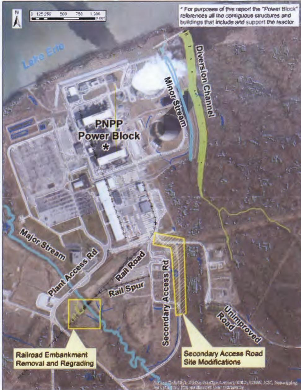
**Figure 3.6.1** Perry Nuclear Power Plant with proposed layout of site modifications. (Source: FENOC Audit –Licensee generated figure, See Section 4) (Source: Public Meeting held June 29, 2017 (ADAMS Accession No ML17193A419))
