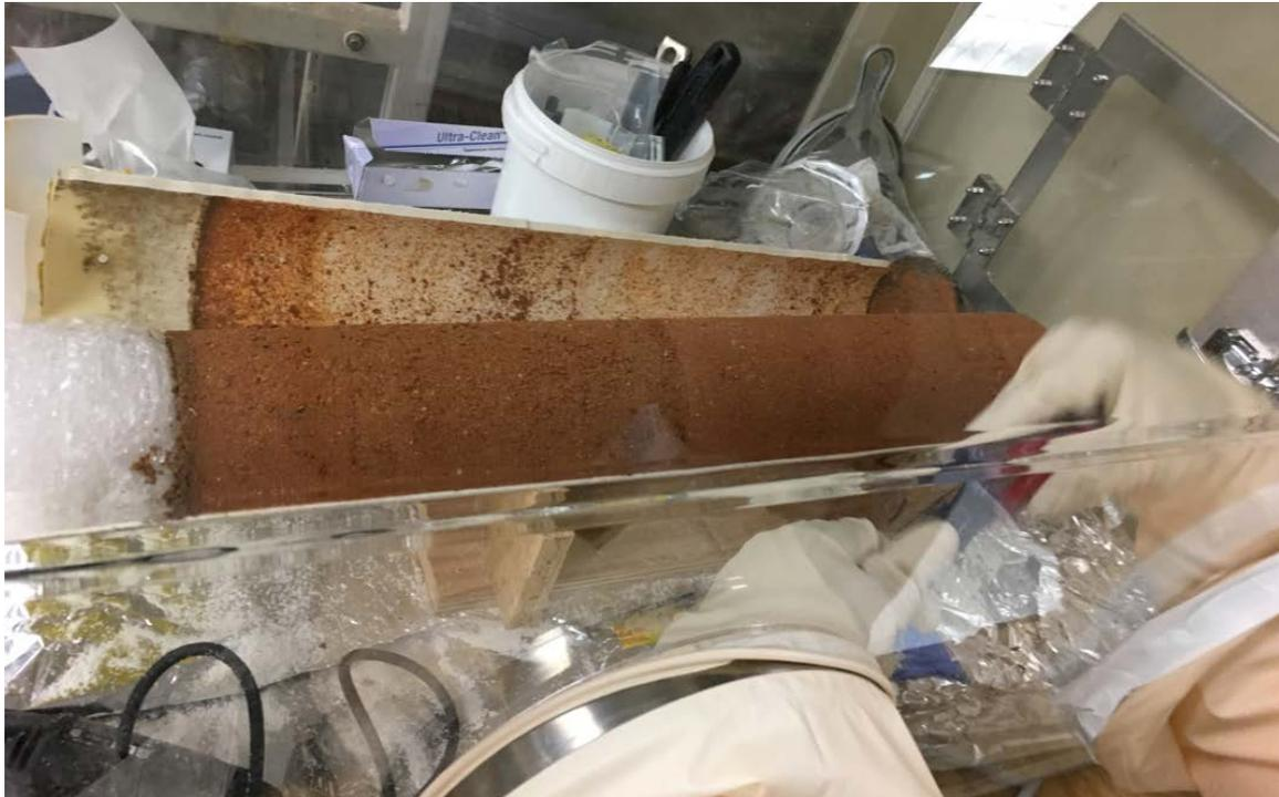
Figure 1. Photograph of intact soil lysimeter #44 in glove box, after removal of top half of PVC containment.
