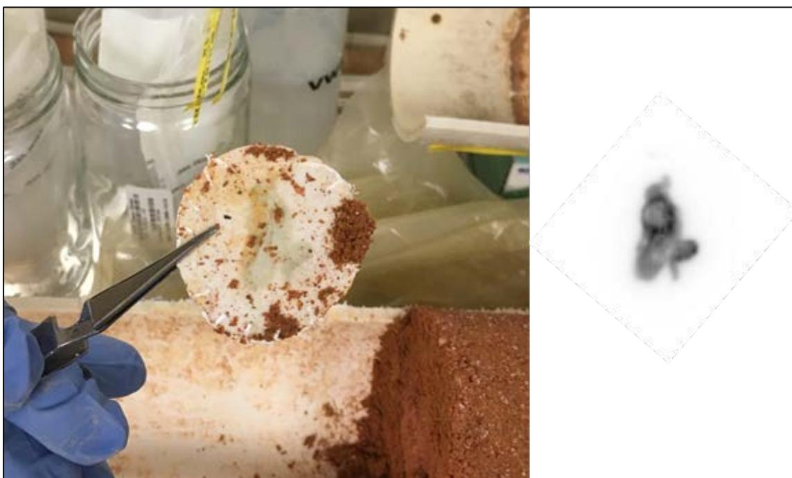
Figure 3: Picture (left) and autoradiography image (right) of lysimeter 44 source. Images are to scale.
