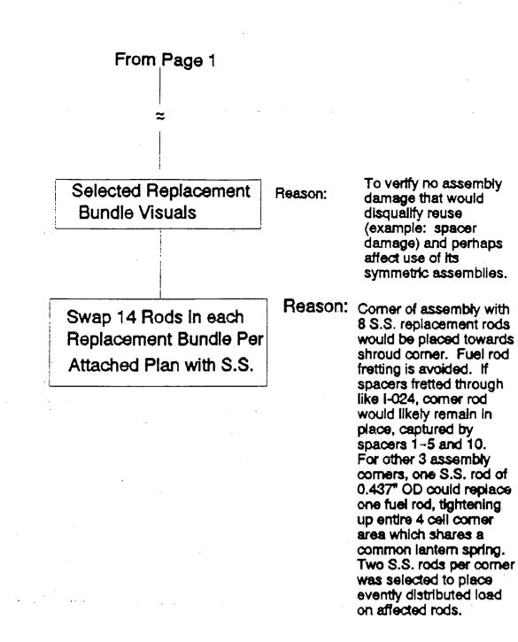
In parallel with the above activities, Pages 3&4 provides inspection items which pertain to root cause investigation of either I-024 failed rod event and/or UGS/SAN-08 stuck bundle event. Root cause inspection items are prioritized above the remedial action of replacement bundles when possible.
