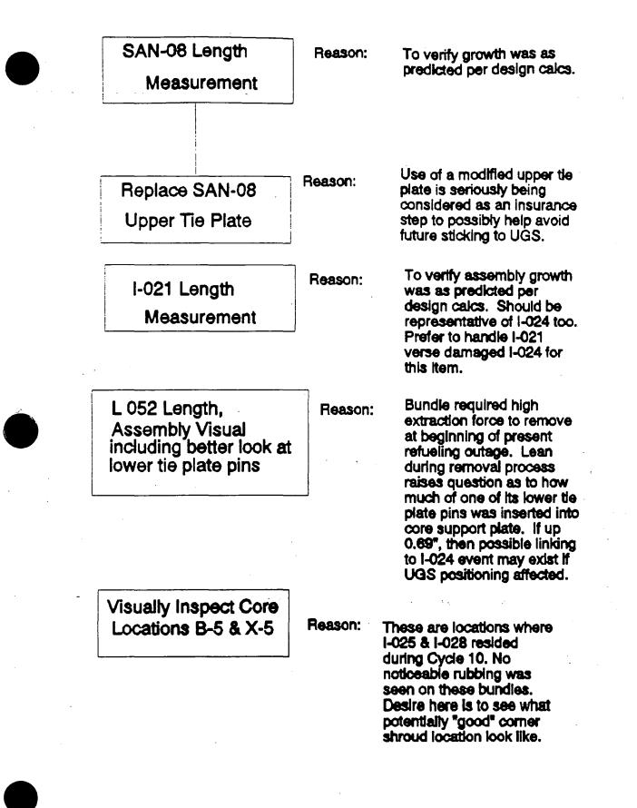
Assembly Visuals on Remaining 10 I-Hf Assemblies When They Are Removed From The Core
