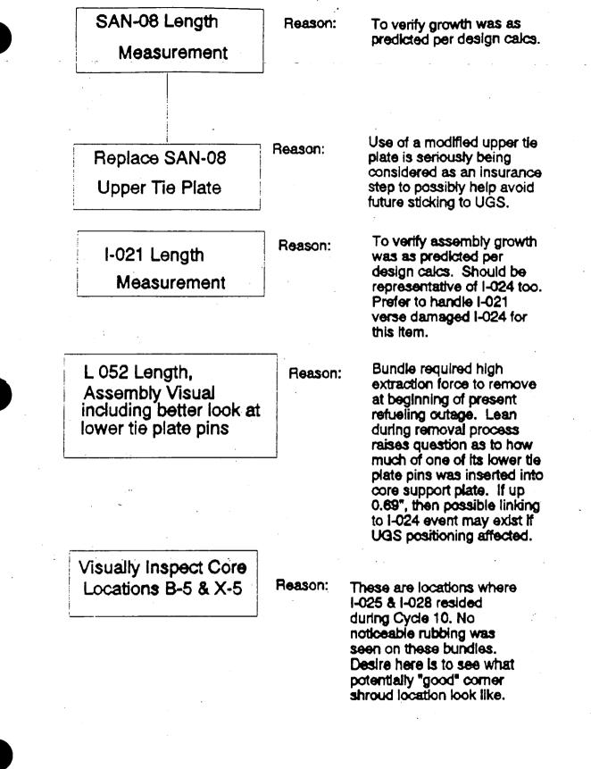
Assembly Visuals on Remaining 10 I-Hf Assembles When They Are Removed From The Core
