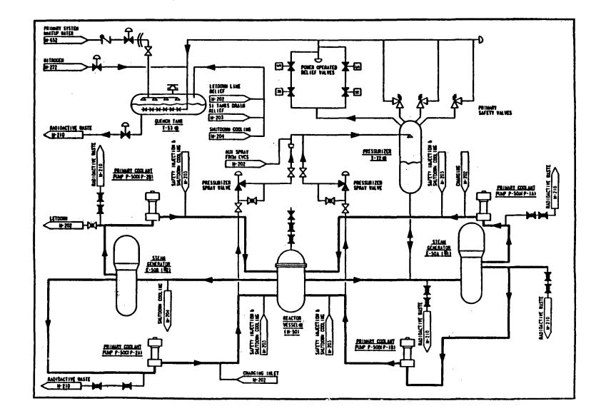
Figure 1.1 Primary coolant system flow
