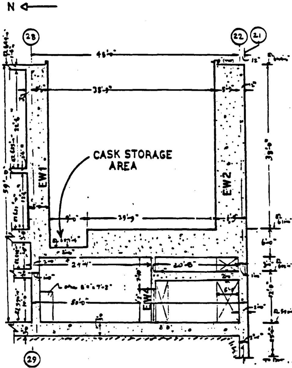
Figure 3-4. Section B-B - Elevation 590 ft to 649 ft
