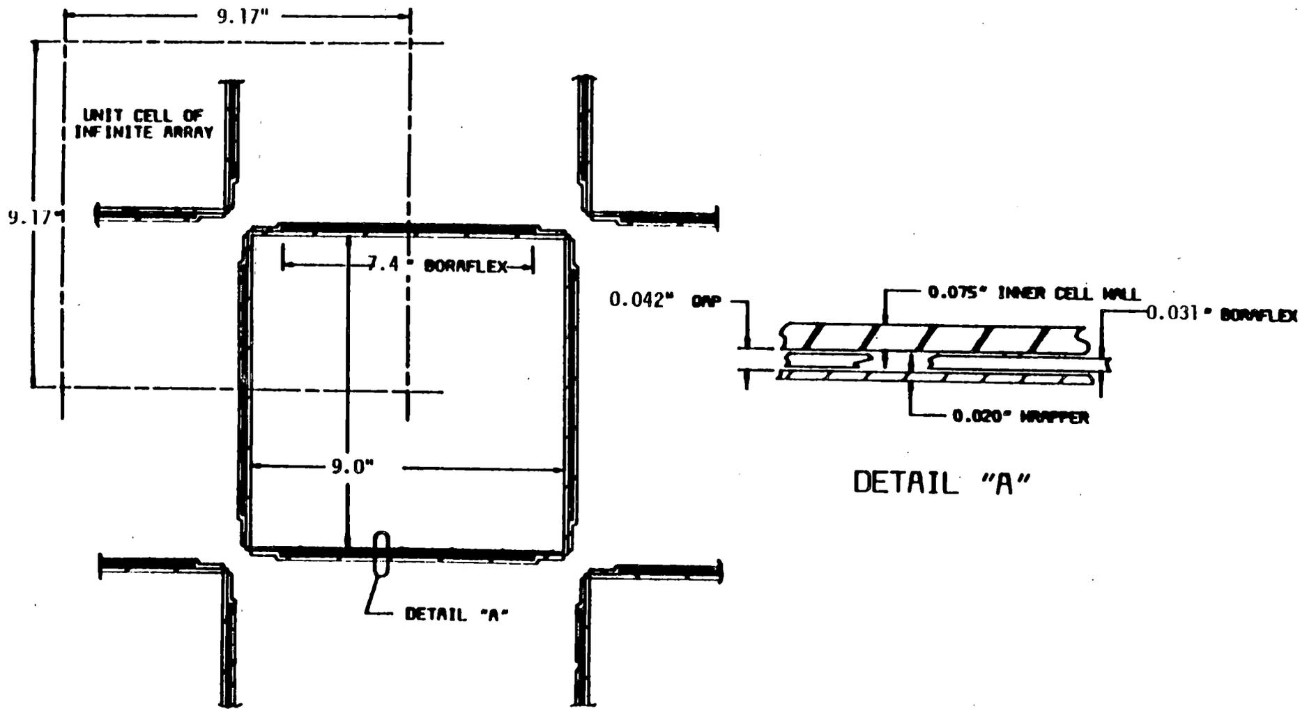
Figure 3-12. Nominal Dimensions for the Region II Storage Cells
