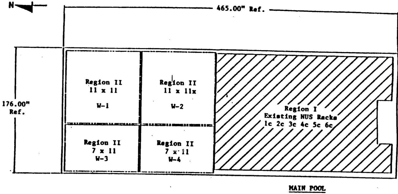
Figure 3-8. Spent Fuel Pool Arrangement
