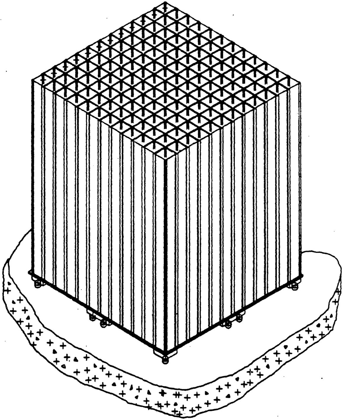
Figure 3-9. Region II Fuel Storage Rack Module
