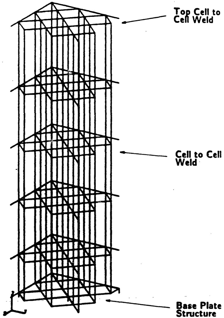
Figure 3-14. Structural Model of Typical Fuel Rack
