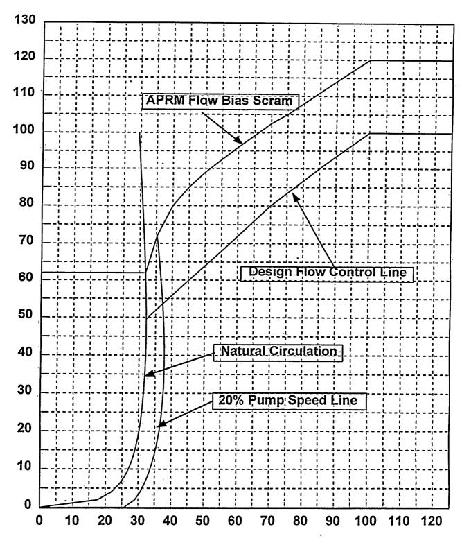
**Core Coolant Flow Rate (% of Design)**
