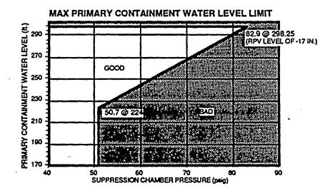
If primary containment water level cannot be maintained below the Maximum Primary Containment Water Level Limit, terminate injection into the Primary Containment from sources external to the primary containment irrespective of whether adequate core cooling is assured.
