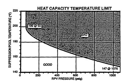
SP/T-3 When suppression pool temperature and RPV pressure cannot be maintained below the Heat Capacity Temperature Limit, EMERGENCY RPV DEPRESSURIZATION IS REQUIRED.
