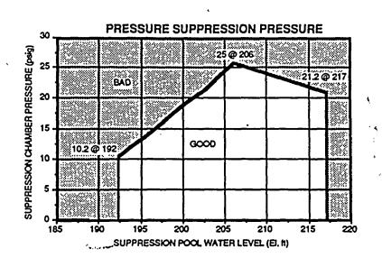
PC/P-3 When suppression chamber pressure cannot be maintained below the Pressure Suppression Pressure, EMERGENCY RPV DEPRESSURIZATION IS REQUIRED.
