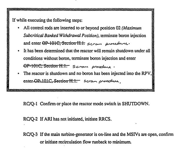
RC/Q-4 If reactor power is above 4% (APRM downseale trip) or cannot be determined, trip the recirculation pumps.
