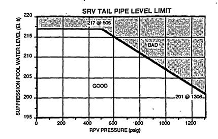
If suppression pool water level cannot be maintained below the SRV Tail Pipe Level Limit, enter RPV Control at Step RC-1 and execute it concurrently with this procedure.
