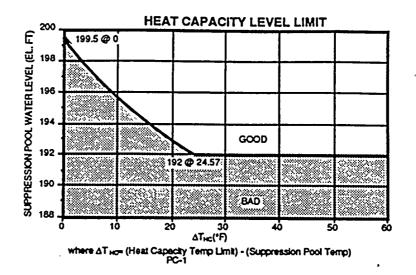
SP/L-2.1 Maintain suppression pool water level above the Heat Capacity Level Limit.
