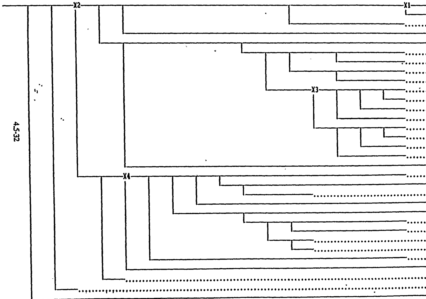
Figure 4.5-3 Nine Mile Point 2 Containment Event Tree for Class I and III Sequences (CET1)
