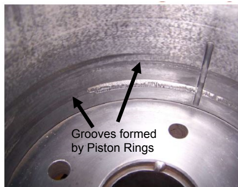
Figure 3: Photo of Grooves Caused by Fretting of Cylinder Wall
