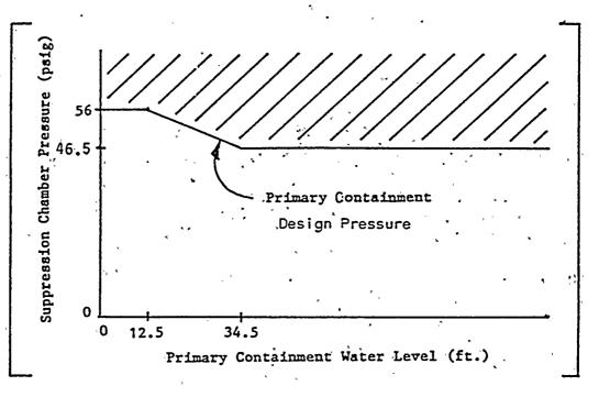
PC/P-6 If suppression chamber pressure cannot be maintained below the Primary Containment Pressure Limit, then irrespective of whether adequate core cooling is assured:
