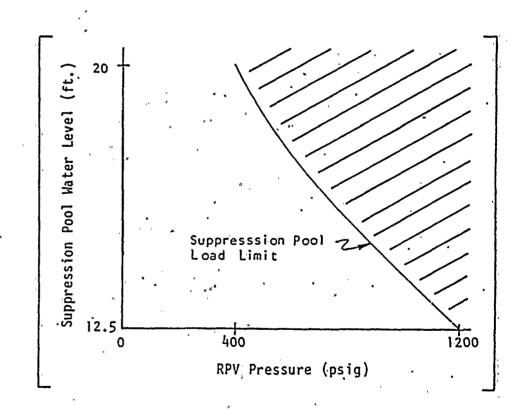
If suppression pool water level cannot be maintained below the Suppression Pool Load Limit, maintain RPV pressure below the Limit. #13 #14
