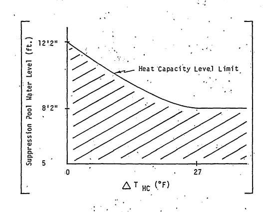
Where  $\Delta T_{HC}$  = Heat Capacity Temperature Limit minus suppression pool temperature
