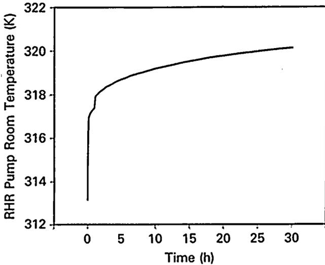
Fig. 1. Simulation of postaccident temperature response within SSES-1 RHR pump room for LOCA on SSES-1 and false LOCA on SSES-2.
