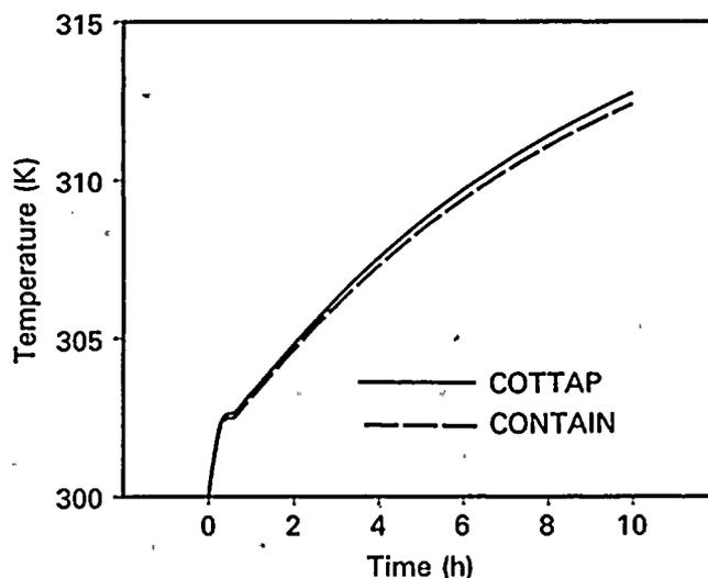
Fig. 5. Comparison of COTTAP and CONTAIN compartment temperature simulations for test problem 1.
