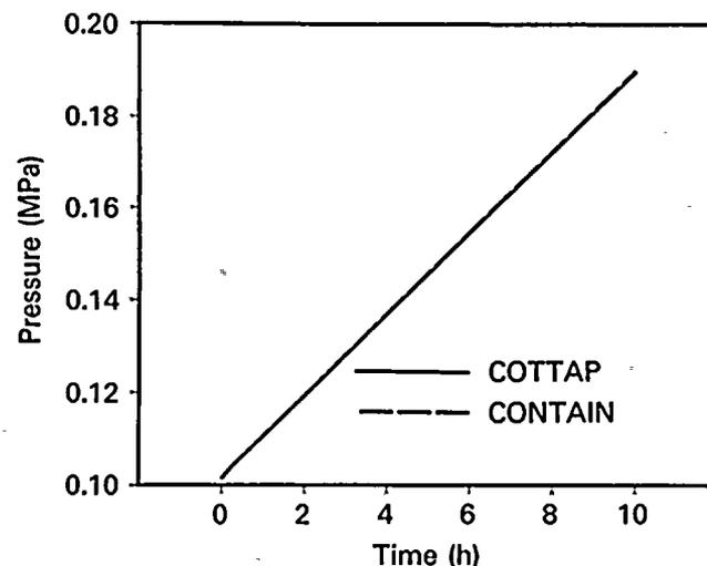
Fig. 6. Comparison of COTTAP and CONTAIN compartment pressure simulations for test problem 1.
