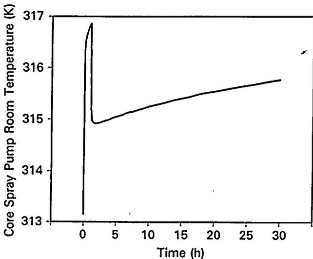
Fig. 2. Simulation of postaccident temperature response within SSES-1 core spray pump room for LOCA in SSES-1 and false LOCA in SSES-2.
