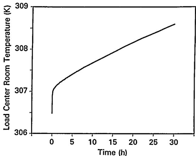
Fig. 4. Simulation of postaccident temperature response within SSES-1 load center room for LOCA in SSES-1 and false LOCA in SSES-2.
