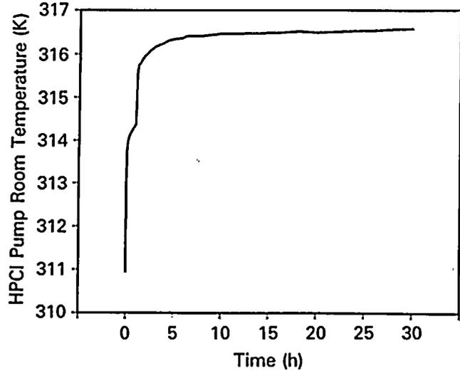
Fig. 3. Simulation of postaccident temperature response within SSES-1 HPCI pump room for LOCA in SSES-1 and false LOCA in SSES-2.
