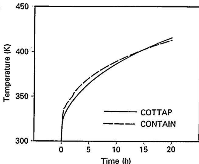
Fig. 7. Comparison of COTTAP and CONTAIN compartment temperature simulations for test problem 2.
