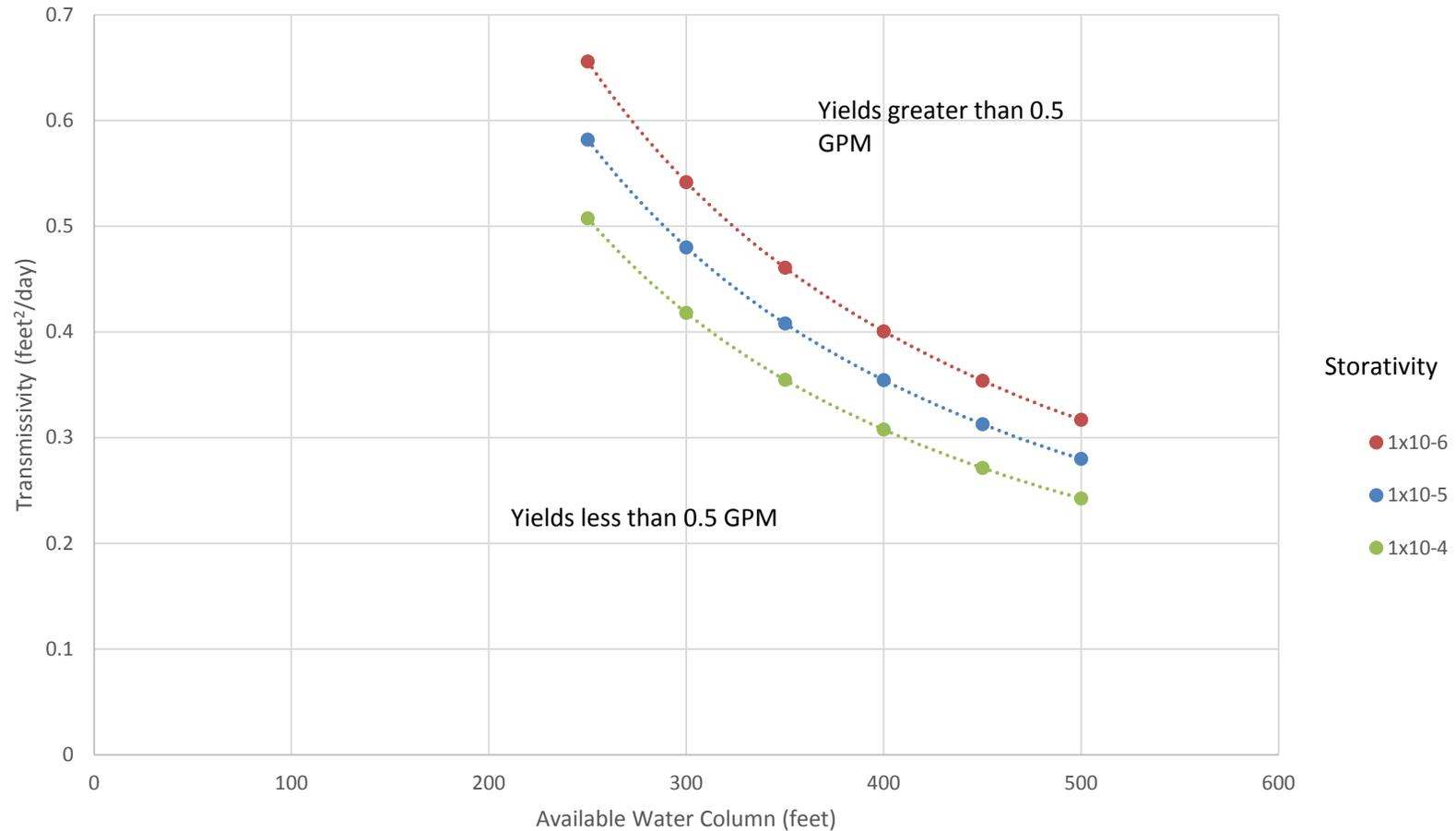
The family of curves depict a well yield of 0.5 gpm for the indicted storativity. Well yields are based on a Cooper-Jacob approximation to the Theis non-equilibrium radial flow to a well. The pumping duration was 365 days and well radius was 0.5 feet.
