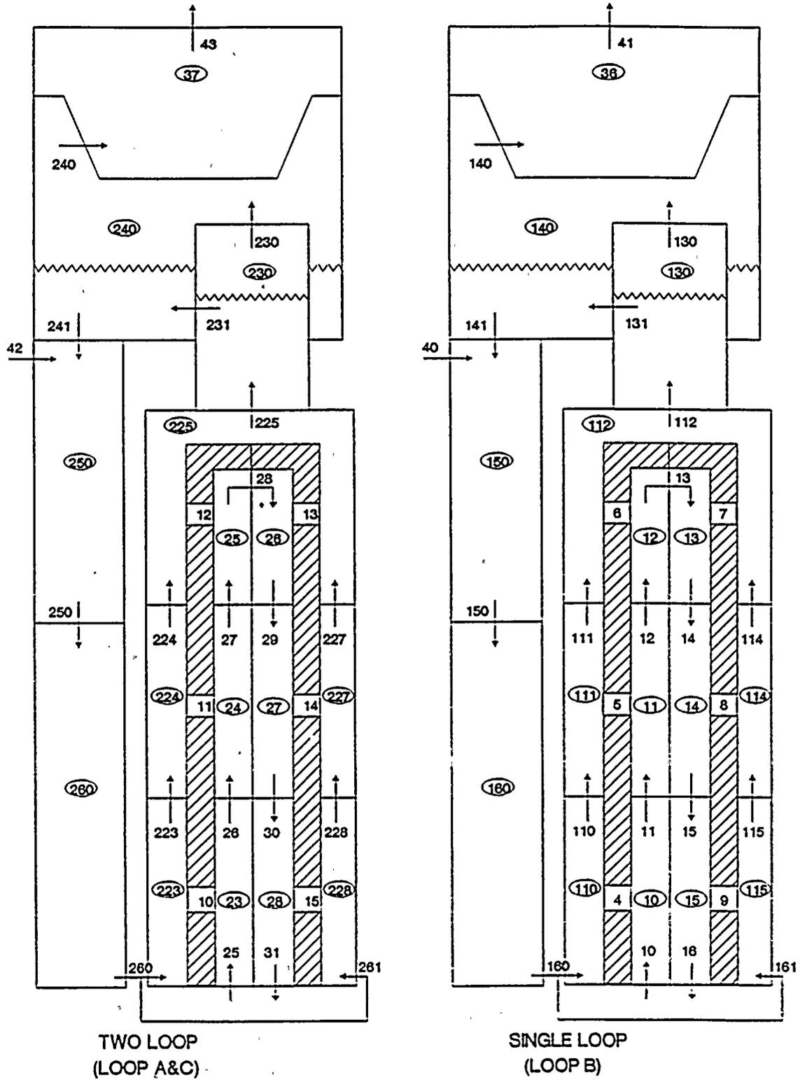
FIGURE 1. TURKEY POINT, RETRAN MULTINODE STEAM GENERATOR MODEL
