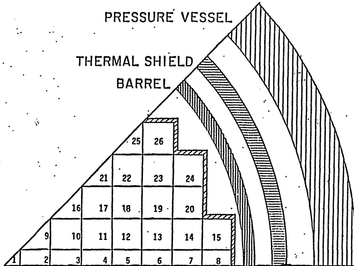
Figure 1 - Turkey Point Geometry Configuration and Assembly Numbering
