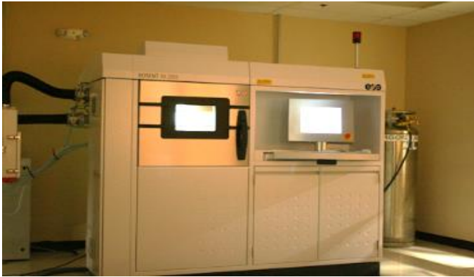
Laser PBF – Open Architecture EWI-Designed and Built
