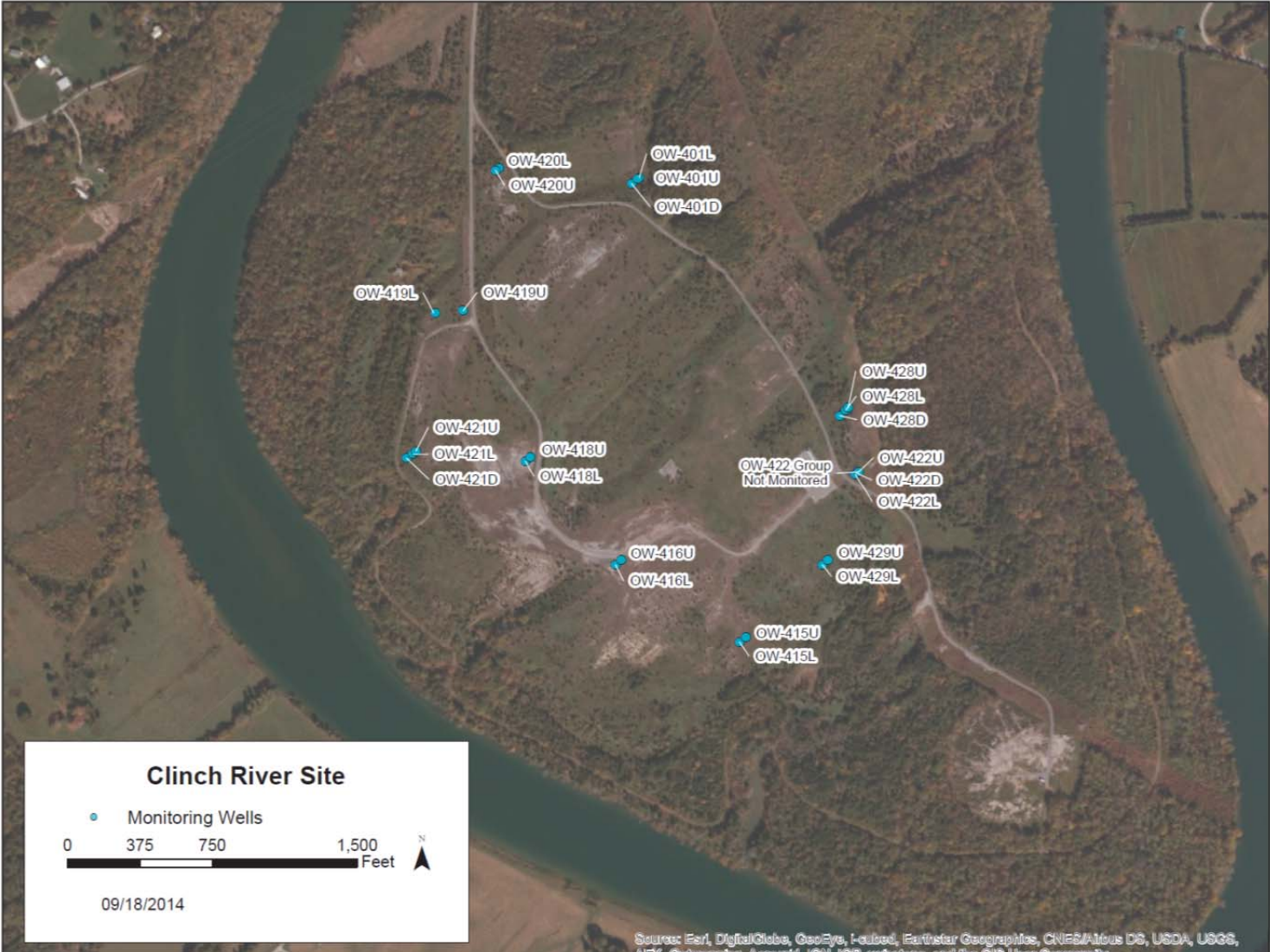
Figure 3: Clinch River Site Groundwater Monitoring Wells
