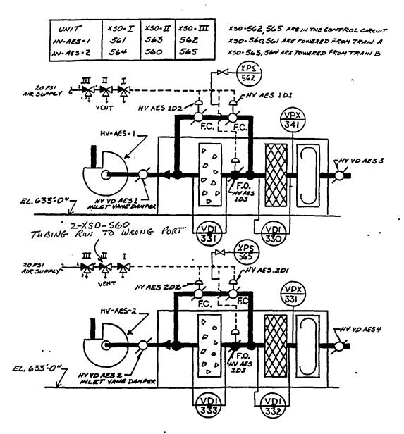
SOLENOIDS I I II TO DE-ENERGIZE ON CONTAINMENT ISOLATION PHASE "B" SIGNAL CAUSING ARE TO FLOW THROUGH FILTER
