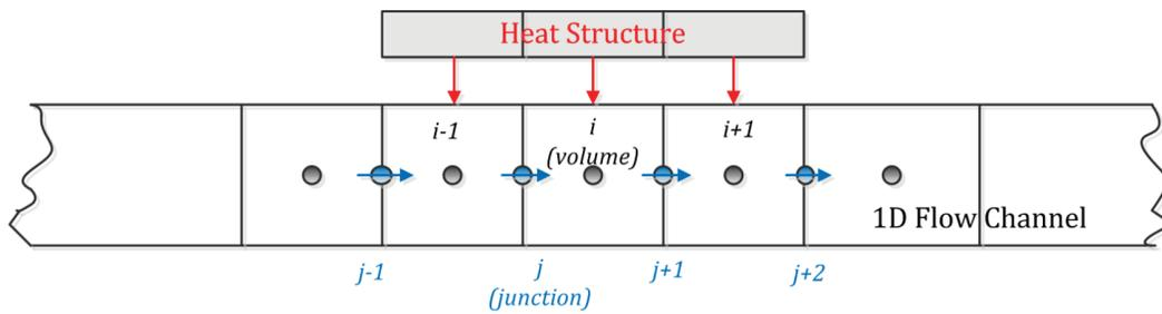
Figure 1. NRELAP5 Staggered Mesh with Heat Structure Coupling
