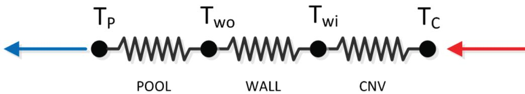
Figure 3. Thermal resistance network between CNV and UHS
