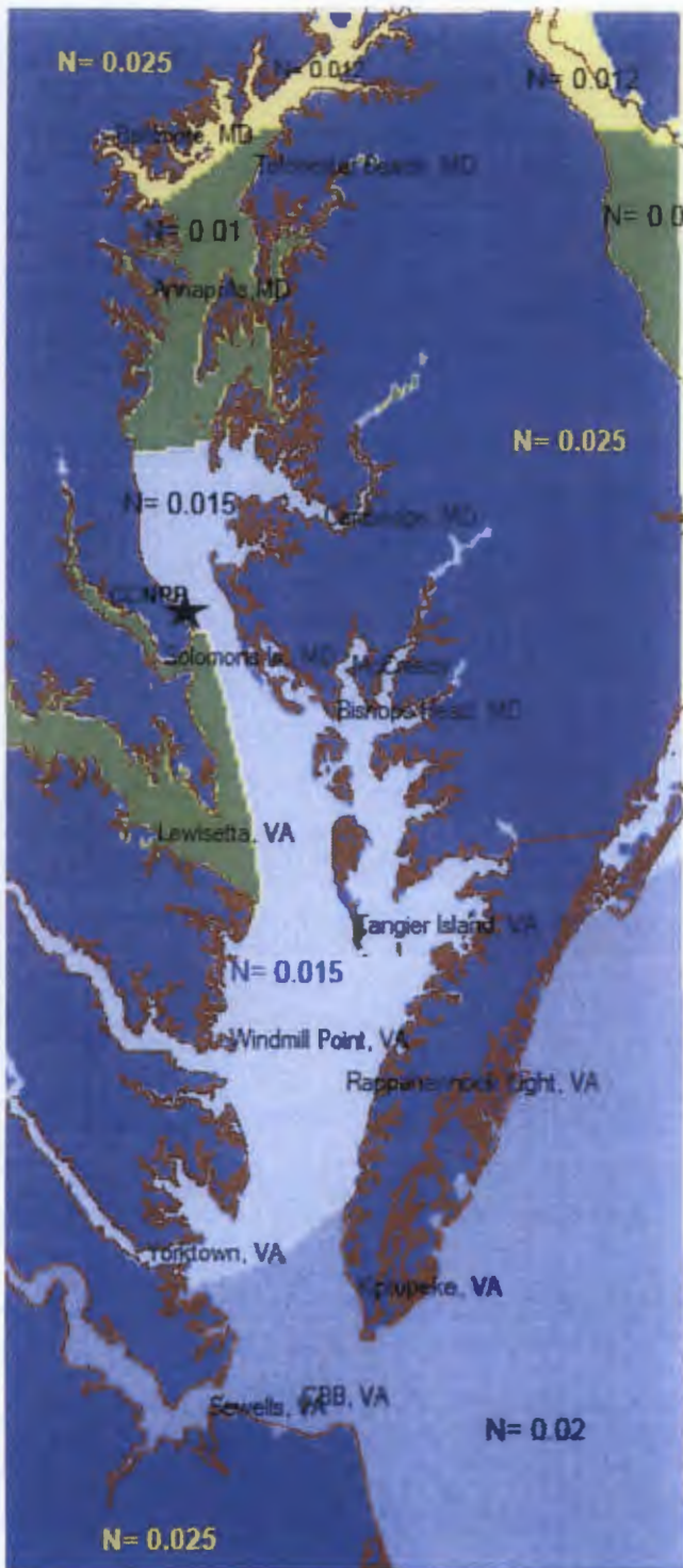
Figure 3.1.2-5. Calibrated Manning's roughness coefficients, or n-values (from the amended FHRR Figure 2.4-16).
