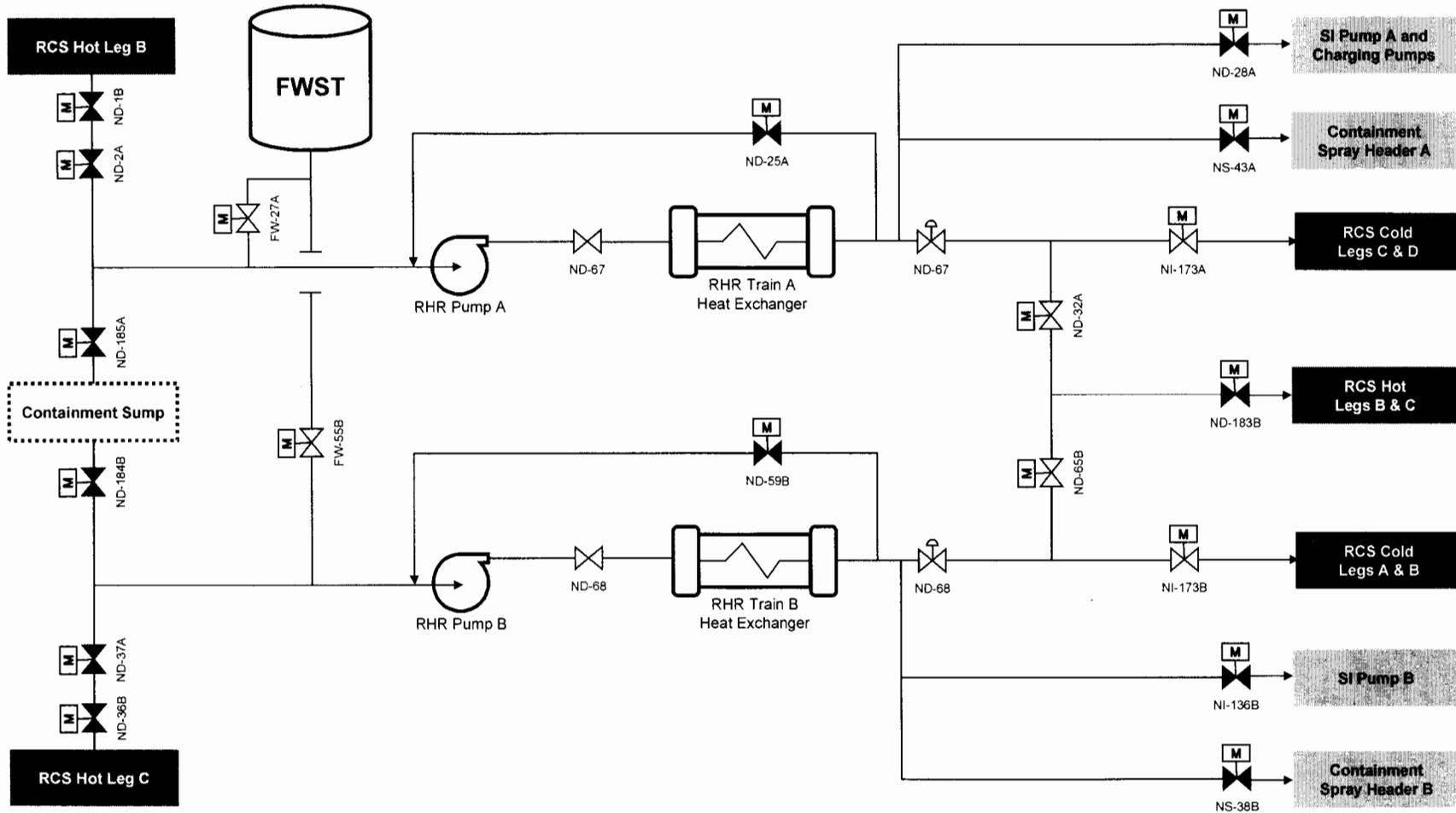
Figure B-1. Simplified RHR System Drawing for Catawba Unit 1
