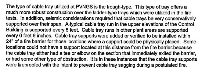
The sections that have a tee or elbow immediately as it exits the barrier have robust construction. The tray sections have a solid bottom, which provides greater structural rigidity over the ladder-type trays that were used in the fire tests. Supports are provided immediately adjacent to the tee or elbow. This structural rigidity and the conservative spacing of the cable tray supports ensures that the fire barrier penetration seal would not fail in the event of a postulated fire.
