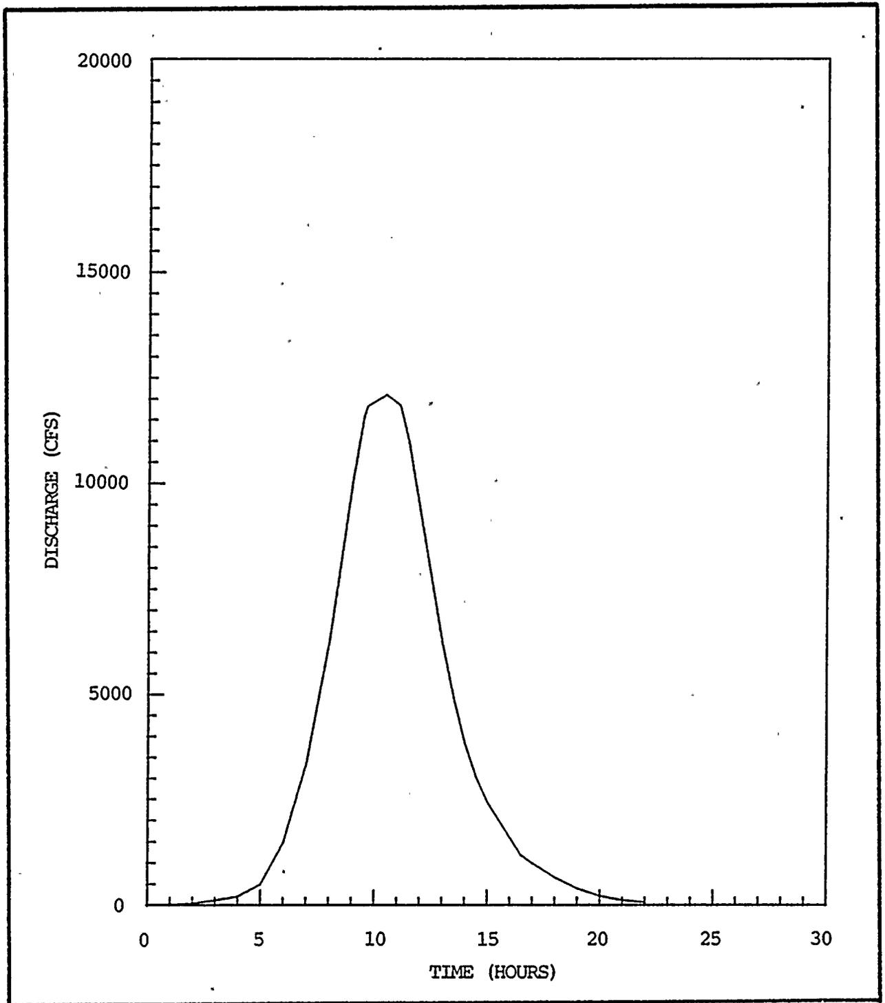
Figure 5 - Deer Creek Flood Hydrograph (24 Hr., 10" Storm)
