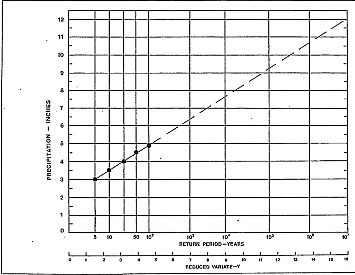
Figure 3 - Return Periods for 24-Hour Precipitations
