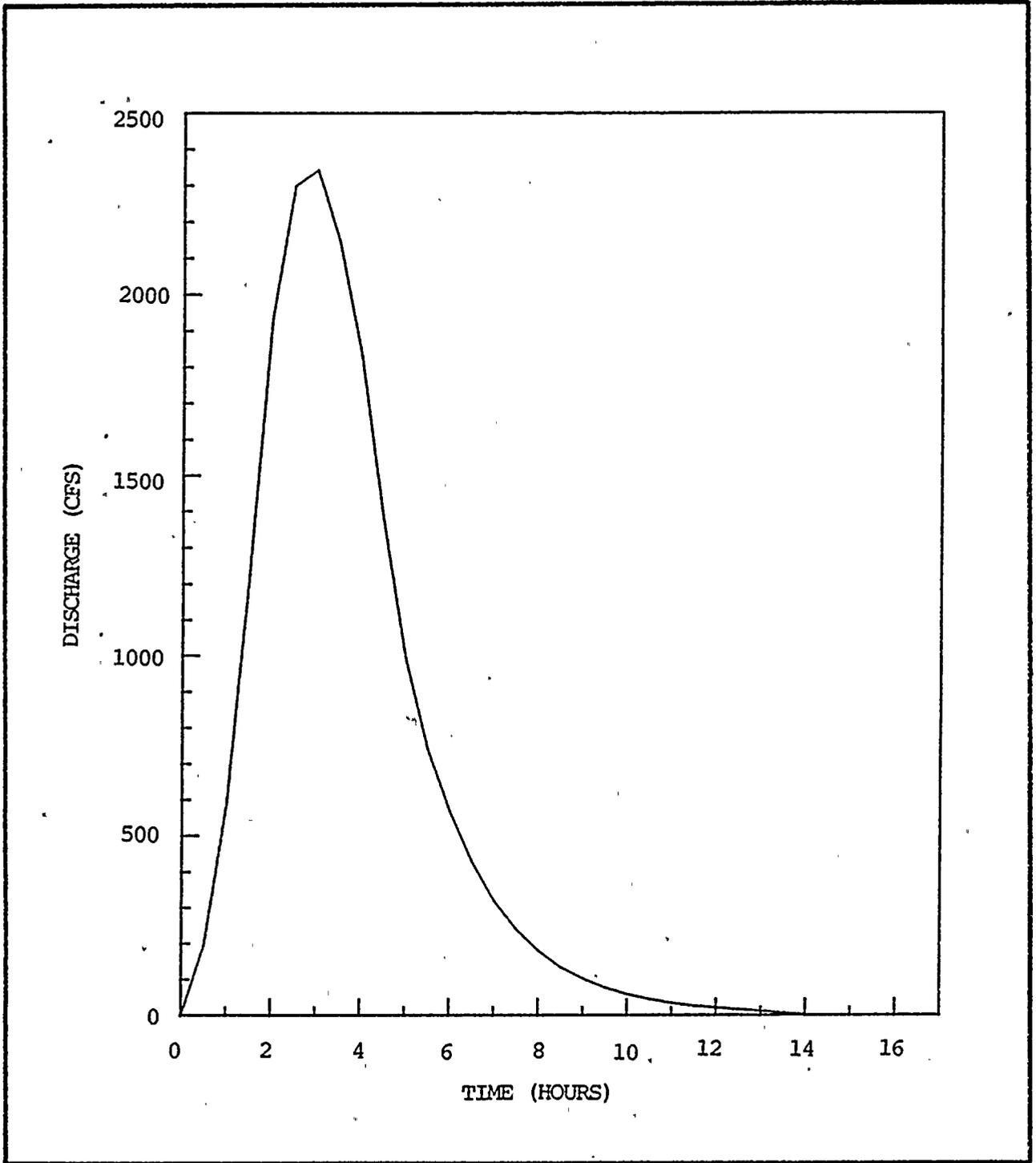
Figure 4 - Unit Hydrograph for Deer Creek (24 Hr., 1" Storm)
