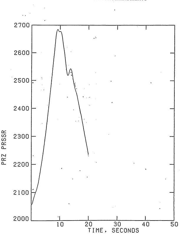
FIGURE 1 RCS PRESSURE vs. TIME FOR LOCV WITH THE PROPOSED TECHNICAL SPECIFICATION AMENDMENTS
