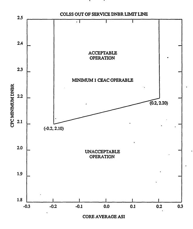
DNBR MARGIN OPERATING LIMIT BASED ON CORE PROTECTION CALCULATORS (COLSS OUT OF SERVICE, CEACS OPERABLE)
