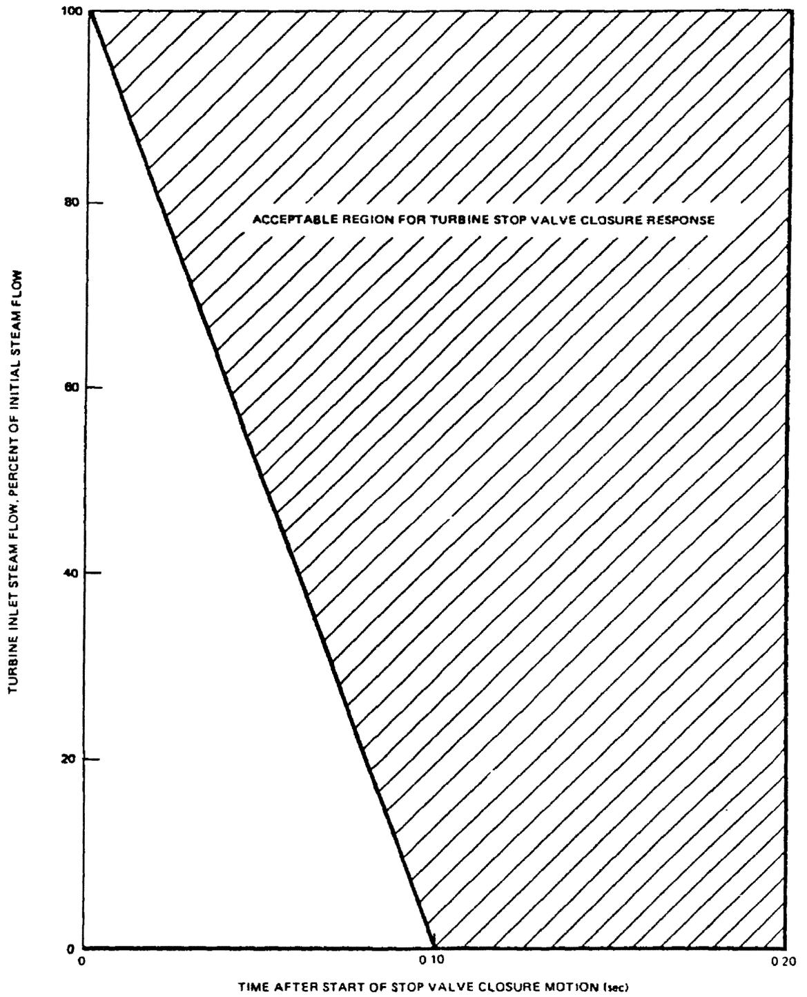
FIGURE 10.2-1. TYPICAL TURBINE STOP VALVE CLOSURE CHARACTERISTIC
