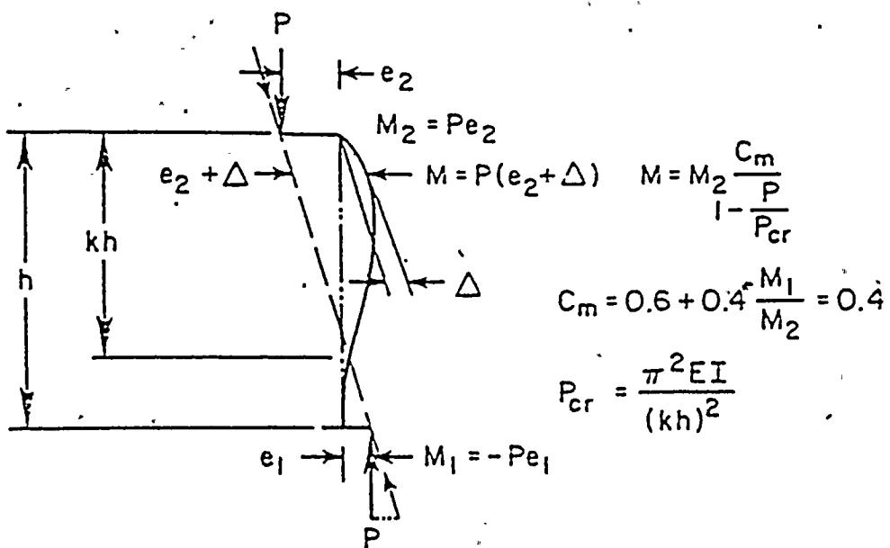
FIG. 4.6 EFFECT OF END CONDITIONS
