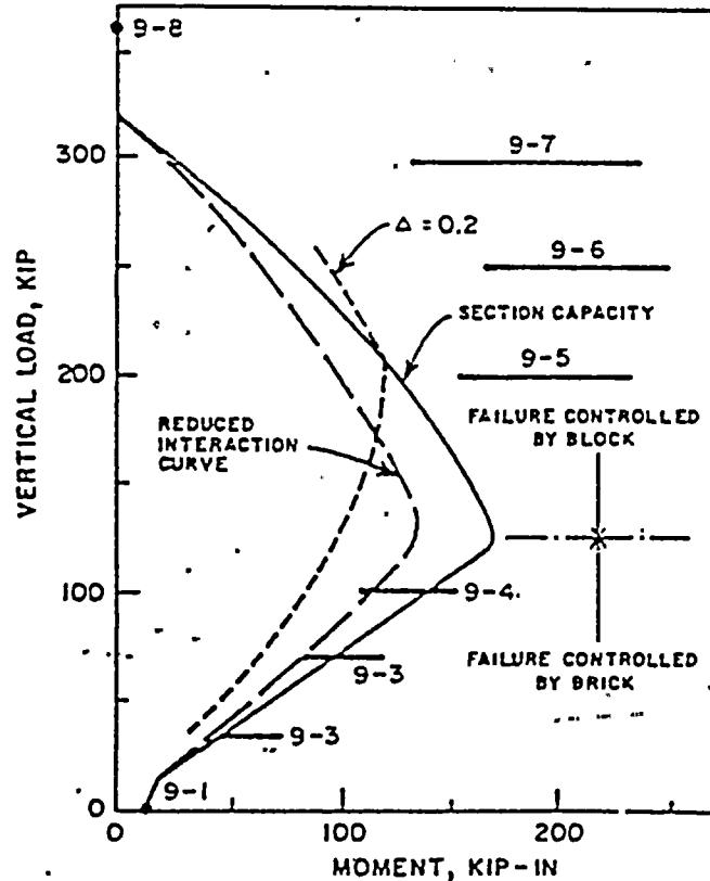
FIG. 4.14 4-2-4 IN BRICK AND CONCRETE BLOCK CAVITY WALLS, CORRELATION WITH PRISM STRENGTH
