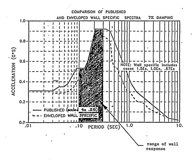
Fig. 1- Floor Spectra at Elevation 74 Ft.
