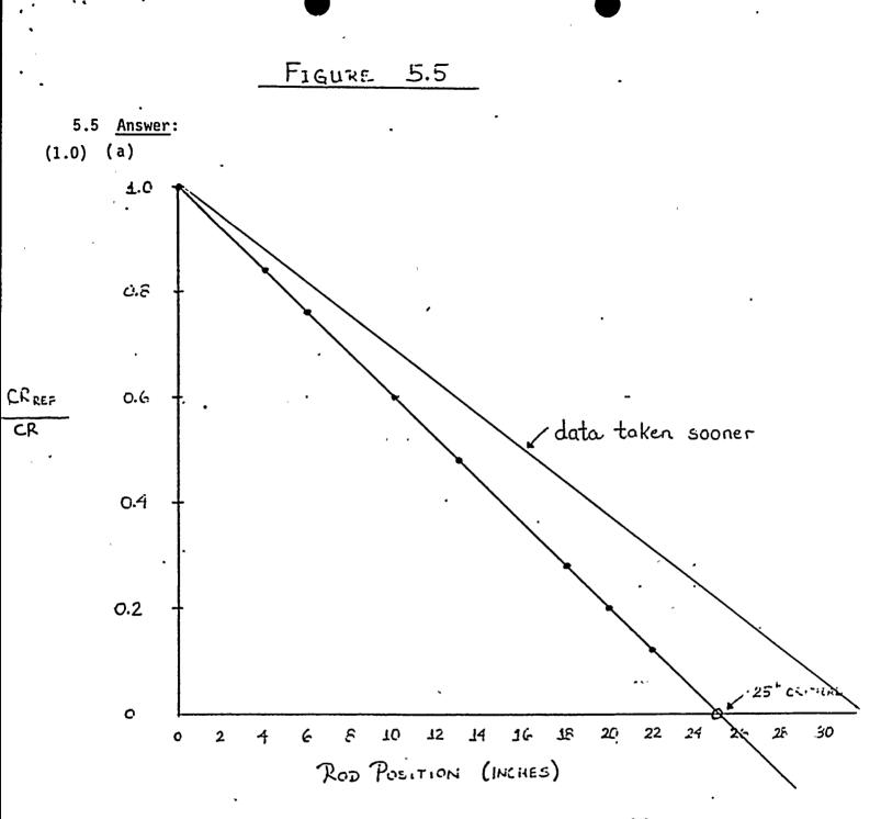
(1.0) (b) If data is taken and plotted too quickly, the count rate will not have increased and stabilized. The plot will show criticality won't be reached until substantial additional rod withdrawal is performed. The operator will not see all the growth in count rate which will yield an estimated critical rod height that is higher than actual critical rod height.
