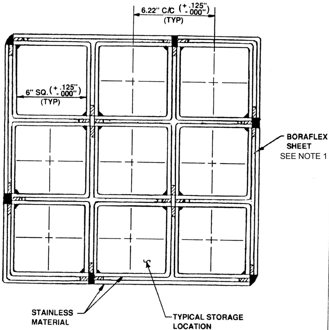
NOTE 1: BORAFLEX SHEETS ARE ABANDONED IN PLACE. NETCO SPENT FUEL POOL RACK INSERTS REPLACE NEUTRON ABSORBING FUNCTION OF THE BORAFLEX SHEETS. (EC 389362)
