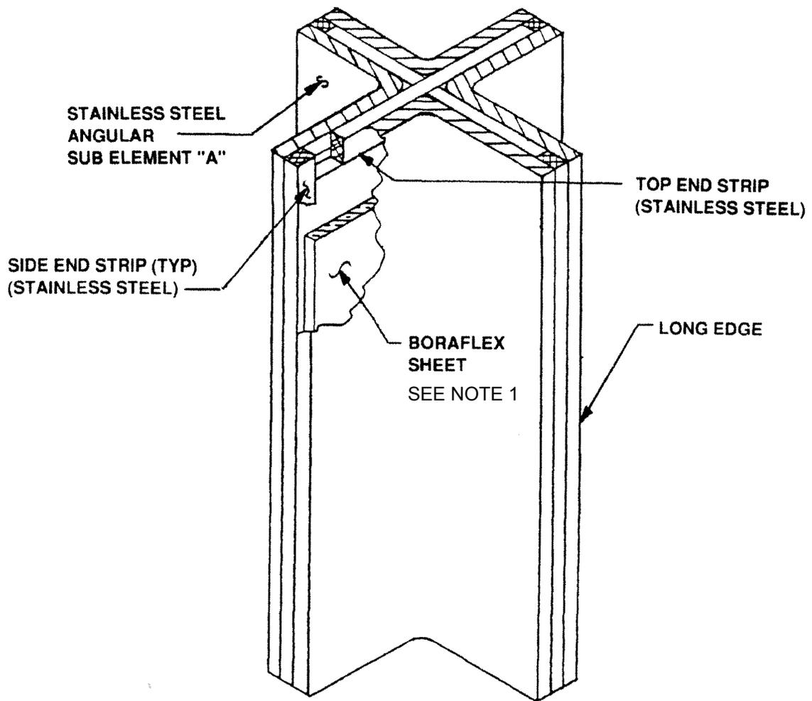
NOTE 1: BORAFLEX SHEETS ARE ABANDONED IN PLACE. NETCO SPENT FUEL POOL RACK INSERTS REPLACE NEUTRON ABSORBING FUNCTION OF THE BORAFLEX SHEETS. (EC 389362)
