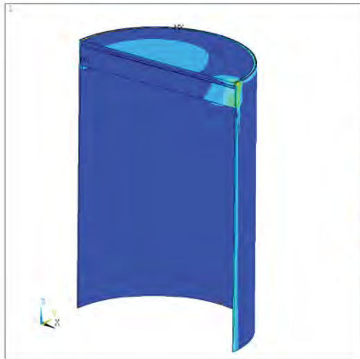
(a) Equivalent (von Mises) Stress [psi] at 75g
