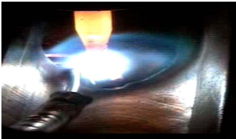
Figure 3-6. Example of dragging filler metal wire resulting in irregular wire entry and weld puddle cooling changes
