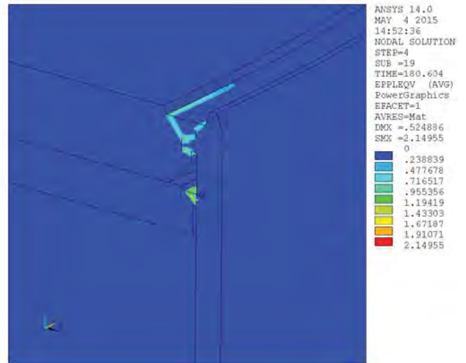
(d) Equivalent Plastic Strain in Weld Region [in/in] at 181g.
