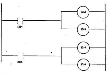
Circuit normally energized Shown in De-Energized Condition
