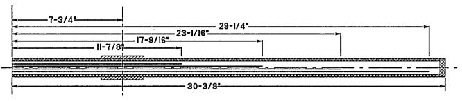
Thermowell is constructed of I" Sch. 80 316 S/S pipe
