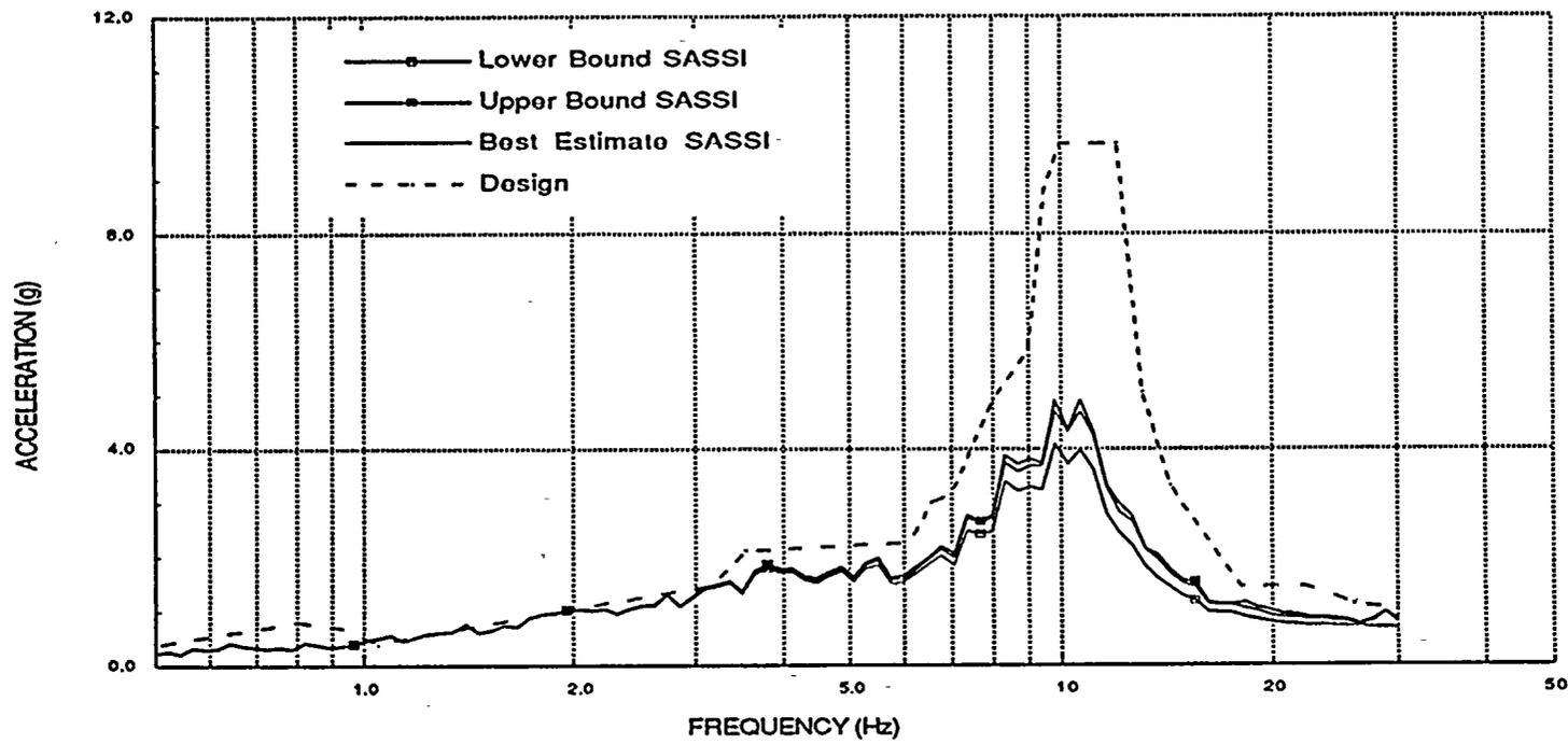
Figure 2.7 - Vertical In-Structure Response Spectra
