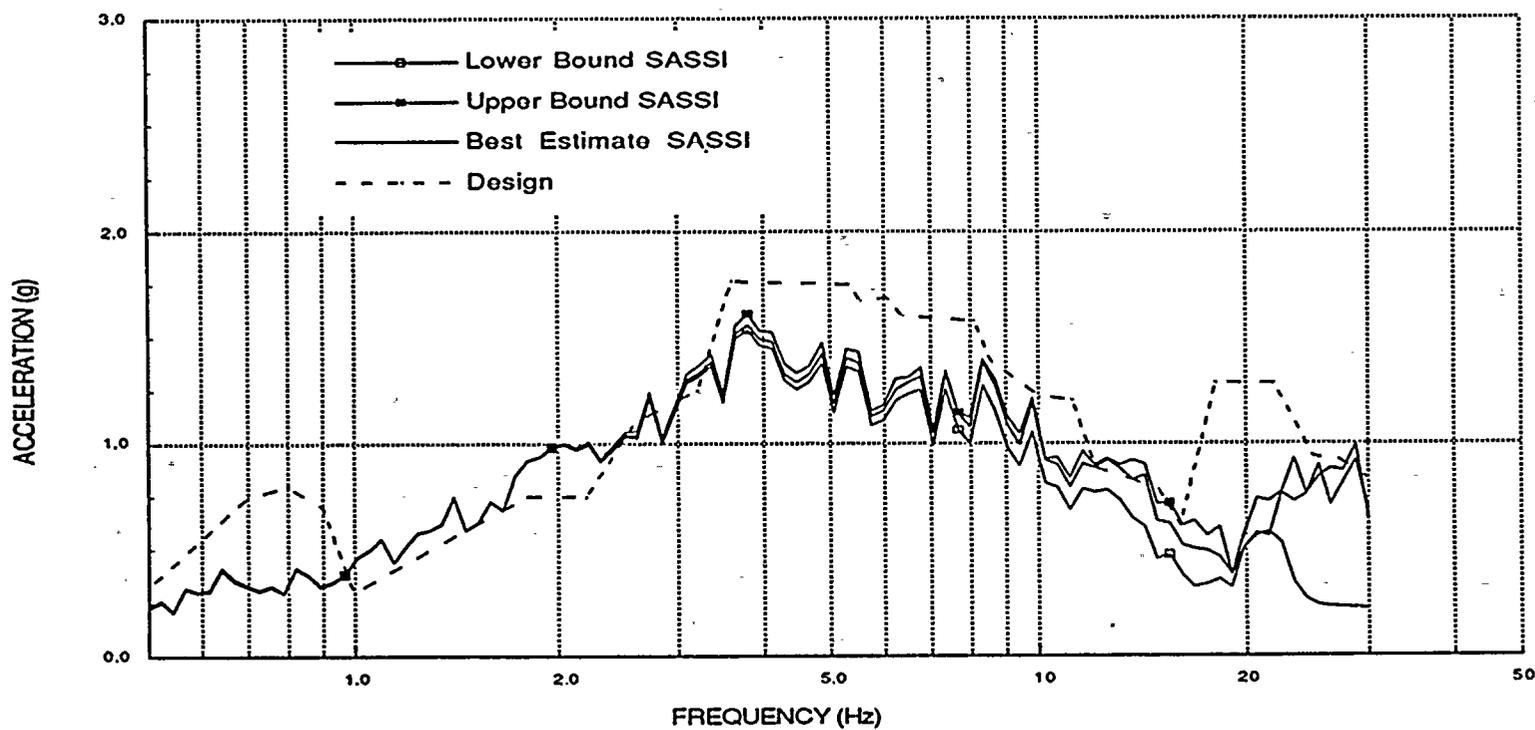
Figure 2.10- Vertical In-Structure Response Spectra
