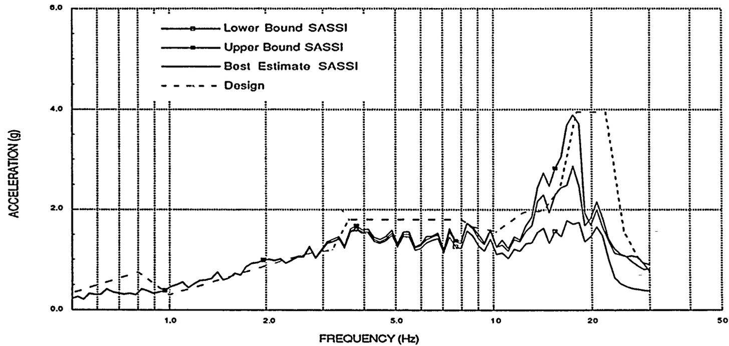
Figure 2.9 - Vertical In-Structure Response Spectra
