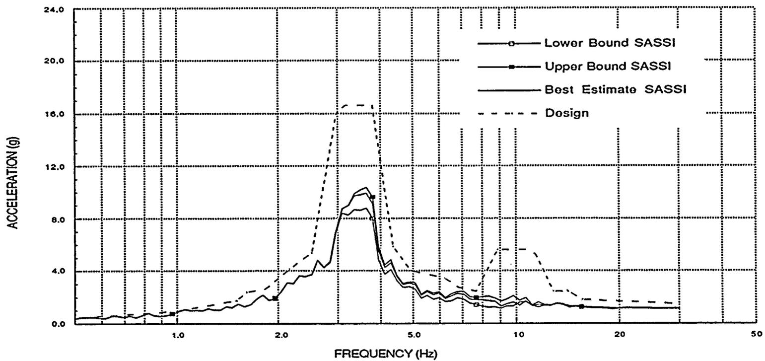
Figure 2.2 - Horizontal In-Structure Response Spectra
