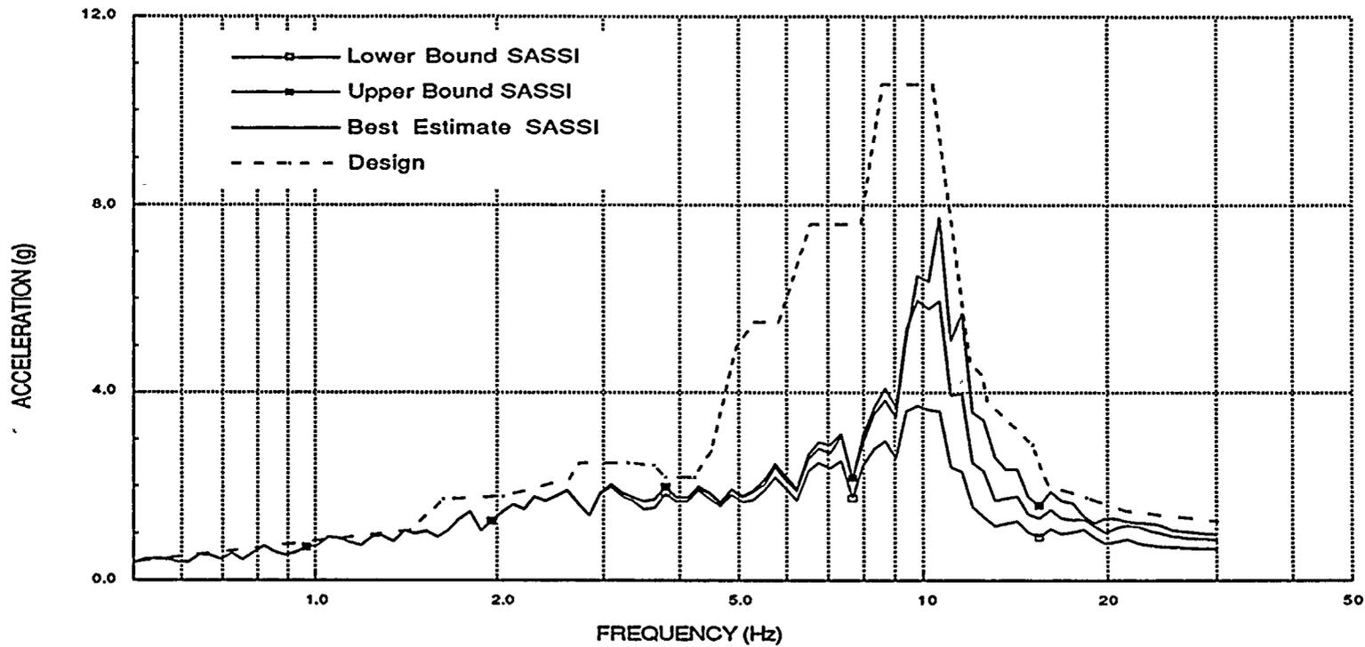
Figure 2.3 - Horizontal In-Structure Response Spectra
