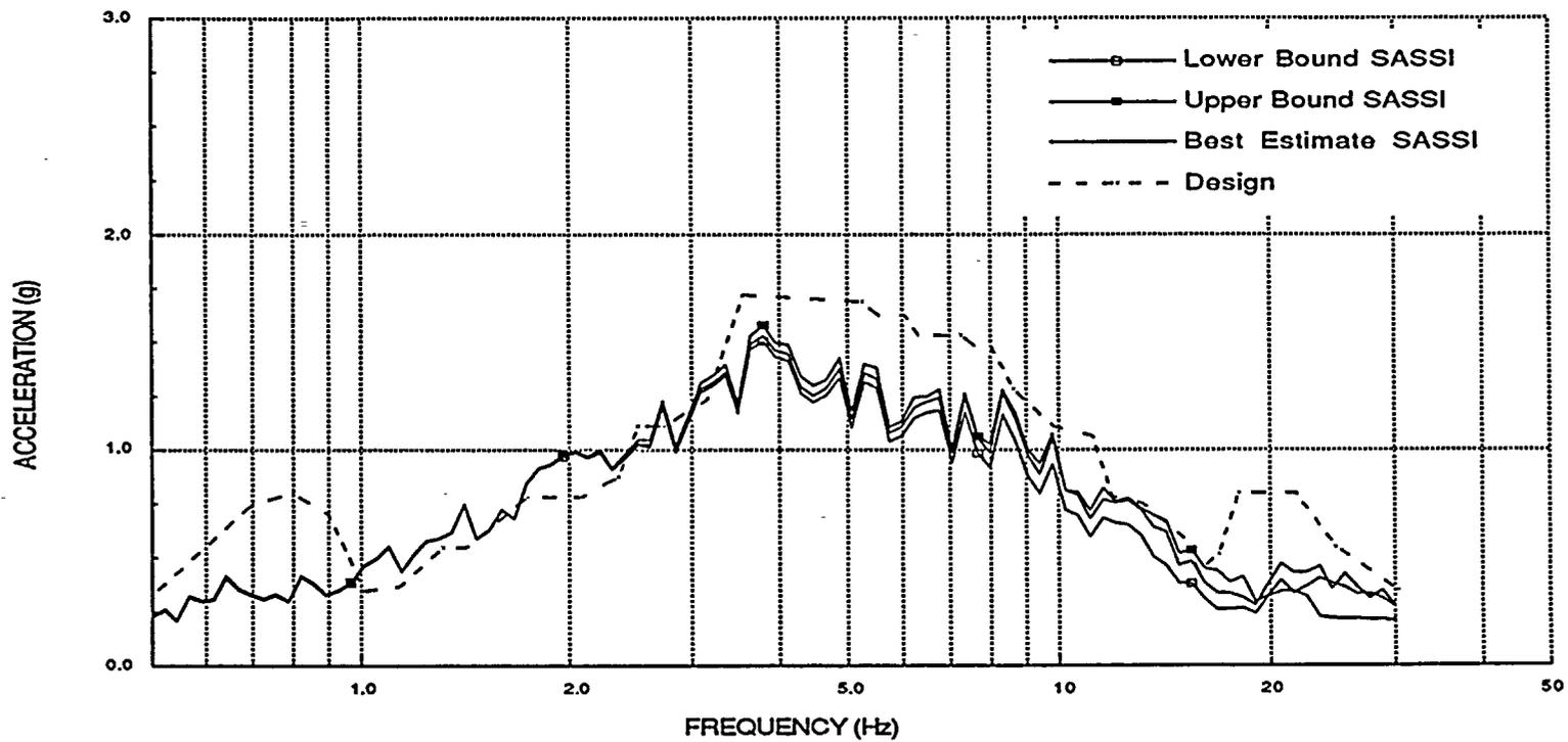
Figure 2.11 - Vertical In-Structure Response Spectra
