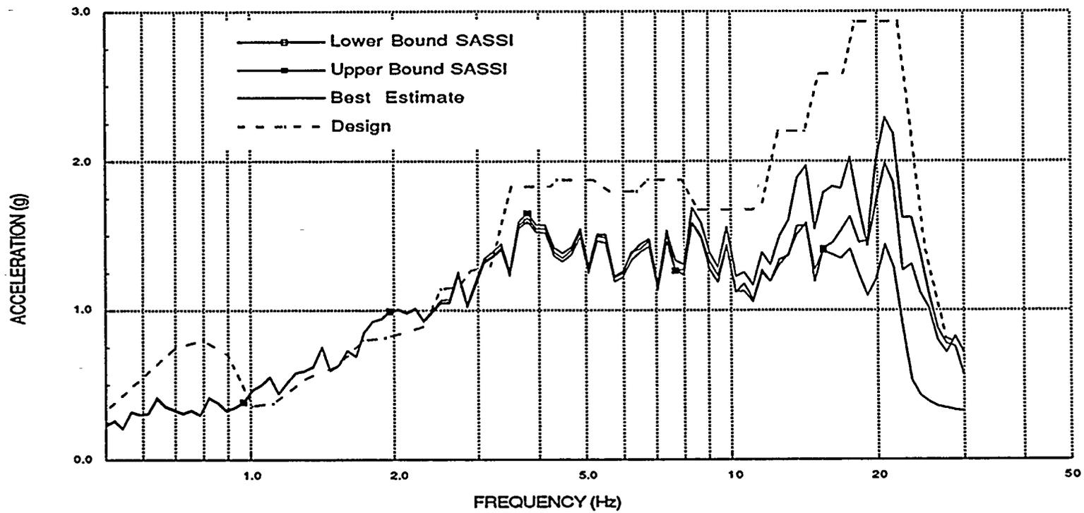
Figure 2.8 - Vertical In-Structure Response Spectra
