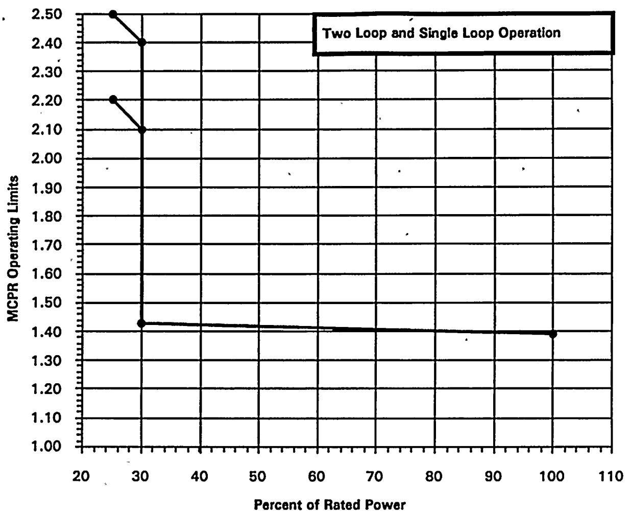
Reduced Power MCPR Operating Limit Versus Percent of Rated Power
