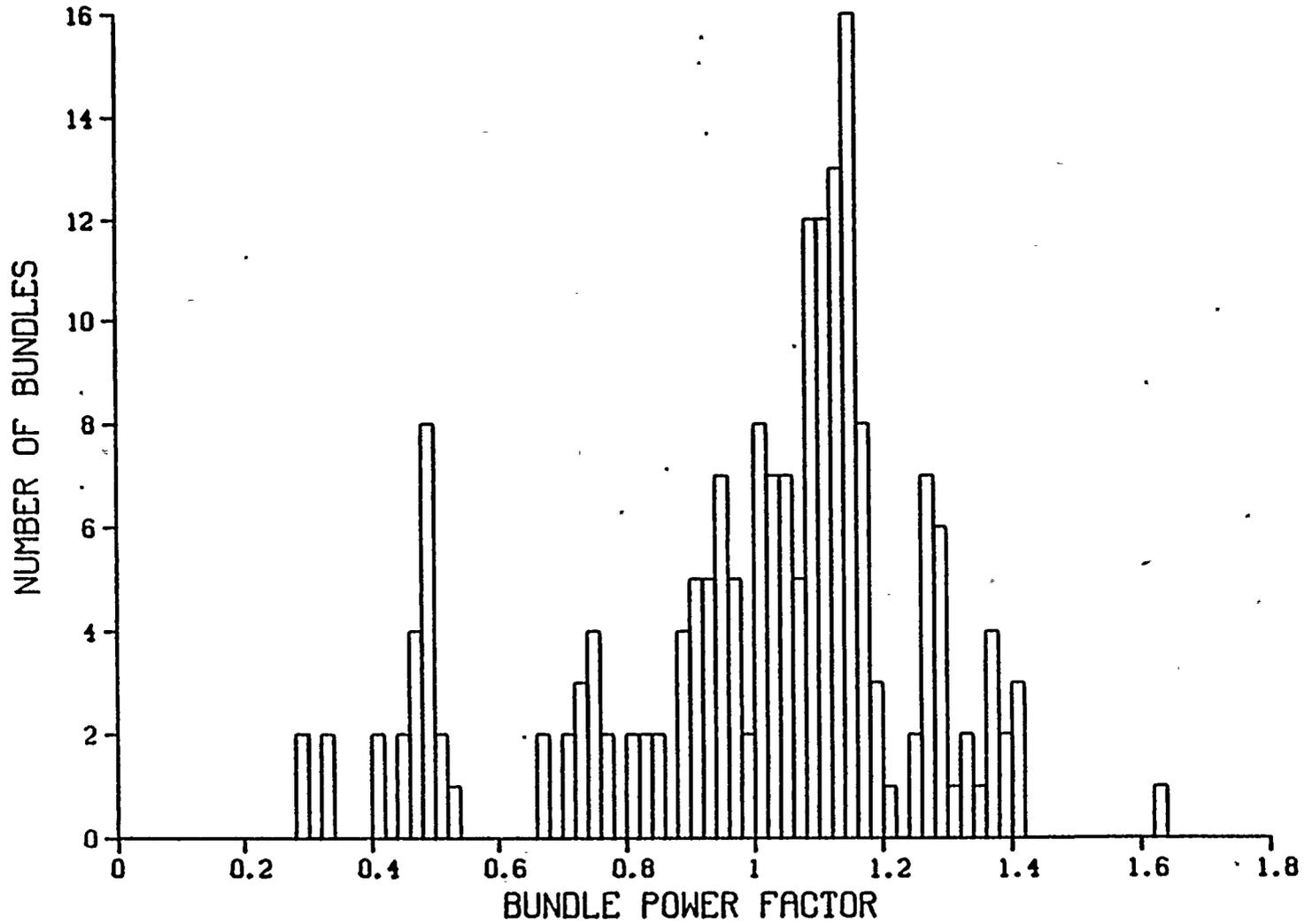
Figure 3.1 Radial Power Histogram For 1/4 Core Safety Limit Model
