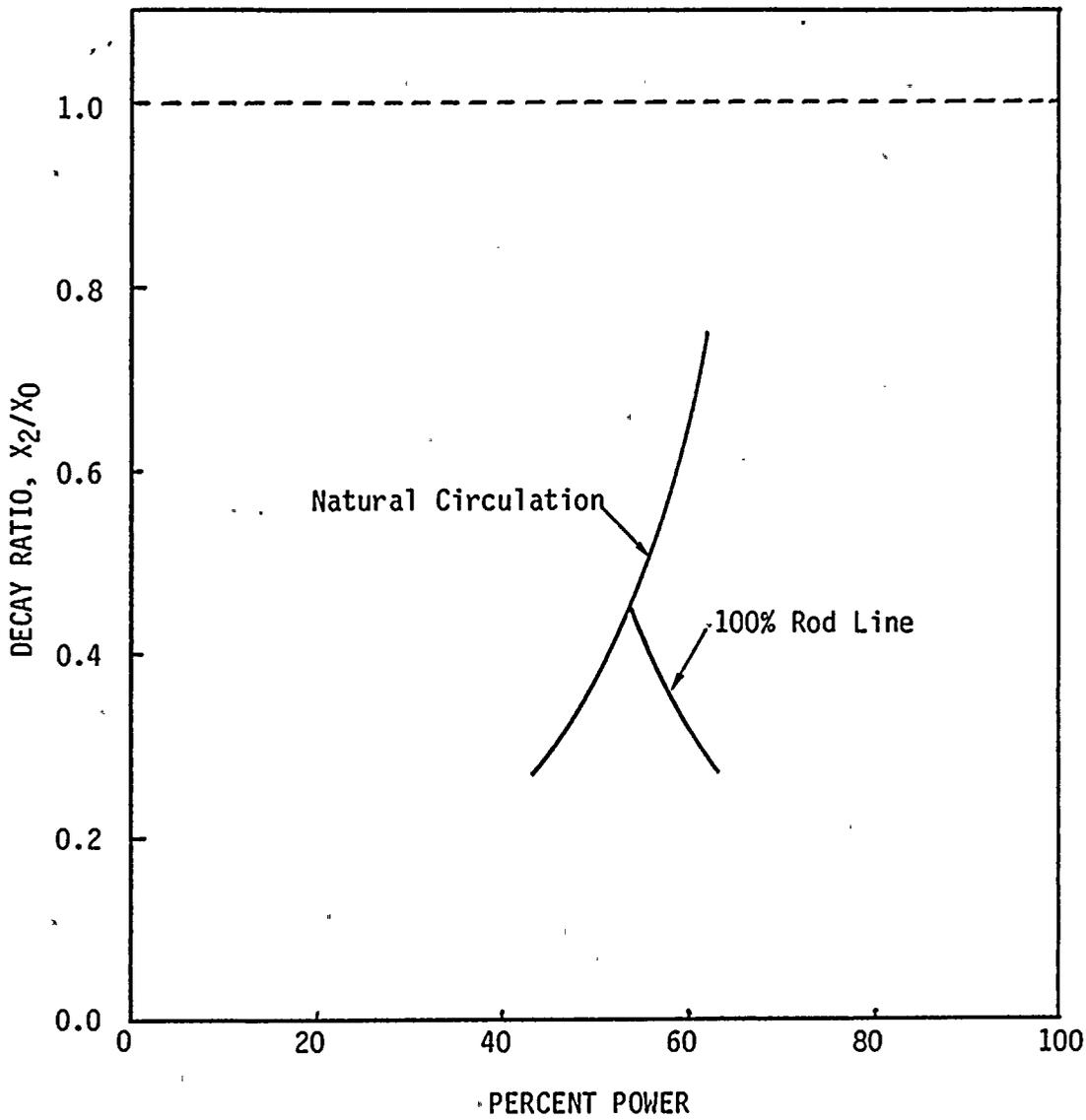
Figure 4.3 Decay Ratio vs. Reactor Power for WNP-2 Cycle 2
