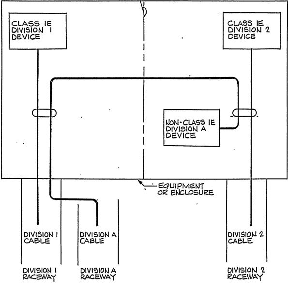
NOTE: SECONDARY BRIDGING IN ENCLOSURES IS ALLOWED WHERE ACCEPTABLE BY ANALYSIS
