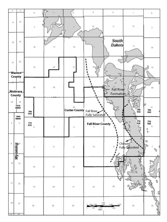
Figure 3.5-7. Map of the Proposed Dewey-Burdock *In-Situ* Recovery Project Area Showing the Approximate Locations of Fully Saturated Portions of the Fall River Formation and Chilson Member of the Lakota Formation. Shaded Areas Are Where Fall River Formation Is Exposed at the Ground Surface. Source: Modified From Powertech (2011)
