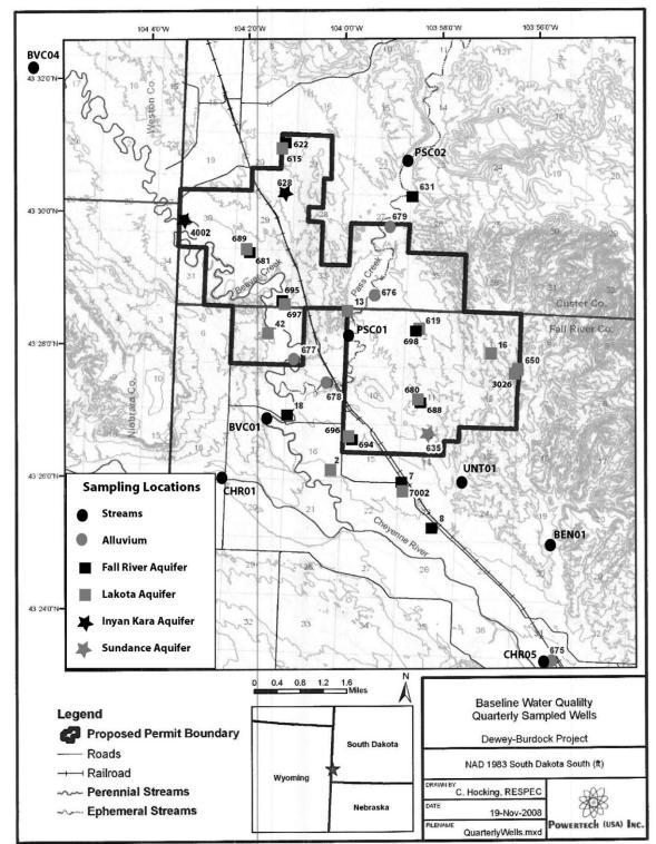
Figure 3.5-2. Map Showing Locations of Beaver Creek, Pass Creek, and the Cheyenne River in Relation to the Proposed Dewey-Burdock *In-Situ* Recovery Project and Water Quality Sampling Locations for Surface Water and Groundwater. Note That Alluvium Samples Were Collected From Wells and Are Not Surface Water Samples.
