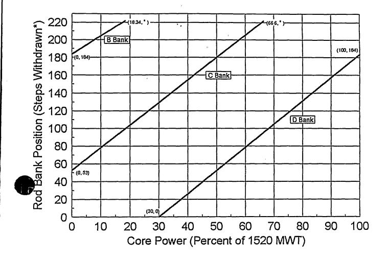
\* The fully withdrawn position is defined as  $\geq$  221 steps.
