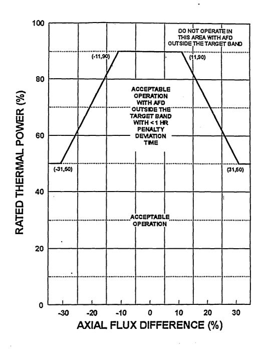
FIGURE 4 AXIAL FLUX DIFFERENCE ACCEPTABLE OPERATION LIMITS AND TARGET BAND LIMITS AS A FUNCTION OF RATED THERMAL POWER
