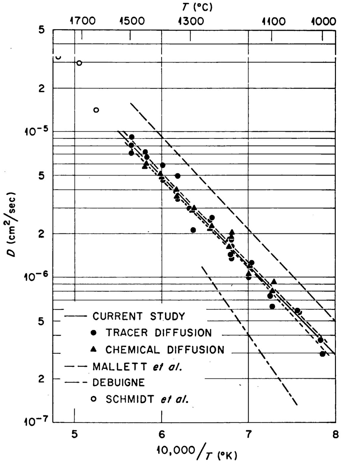
Figure 2. Diffusivity of Oxygen in Beta Phase Zircaloy-4.
