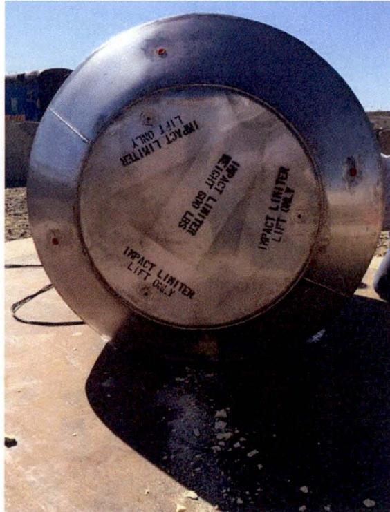
Figure 2.12.3-43 – Impact Limiter-3 after P3 and D3 Free Drop Test
