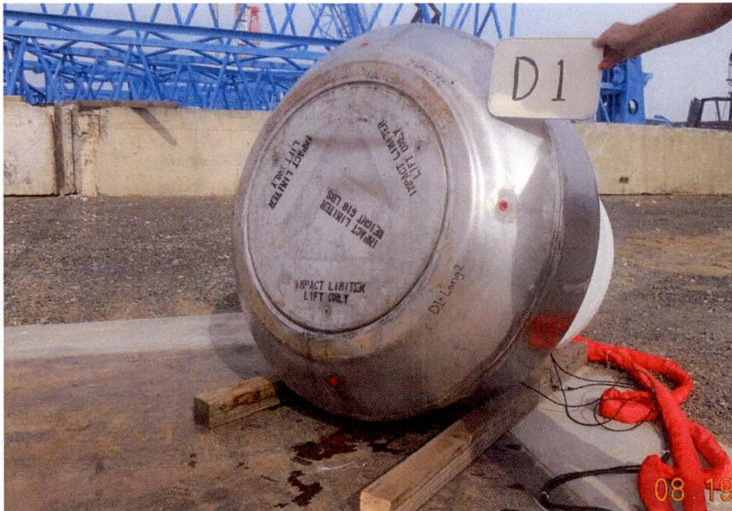
Figure 2.12.3-14 – CTU-1 D1 Damage to Bottom Surface
