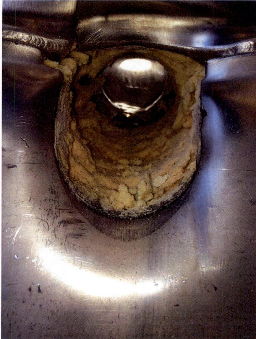
Figure 2.12.3-56 – Impact Limiter-4 Entry Damage after P4 Puncture Drop Test
