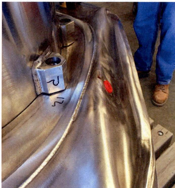
Figure 2.12.3-49 – Impact Limiter-4 Damage after D3 Free Drop Test
