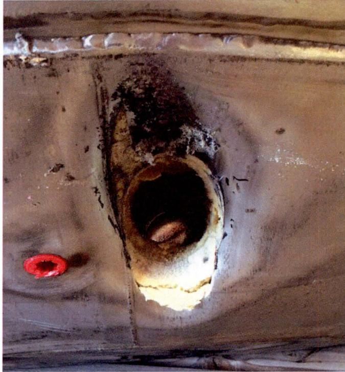
Figure 2.12.3-33 – Impact Limiter-2 Damage after P2 Puncture Drop Test
