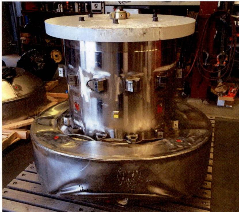
Figure 2.12.3-29 – CTU-2 Damage after P2 Puncture Drop Test
