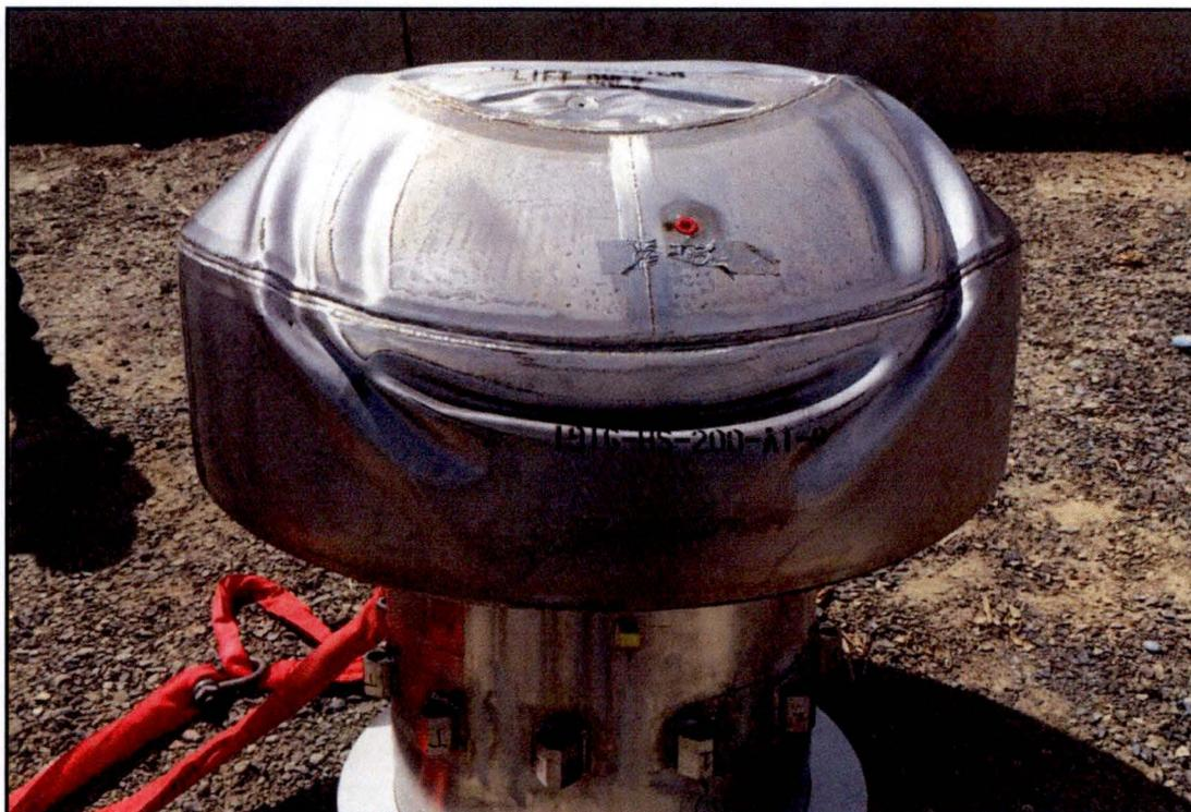
Figure 2.12.5-20 – CTU-2 Damage after D2 Free Drop Test
