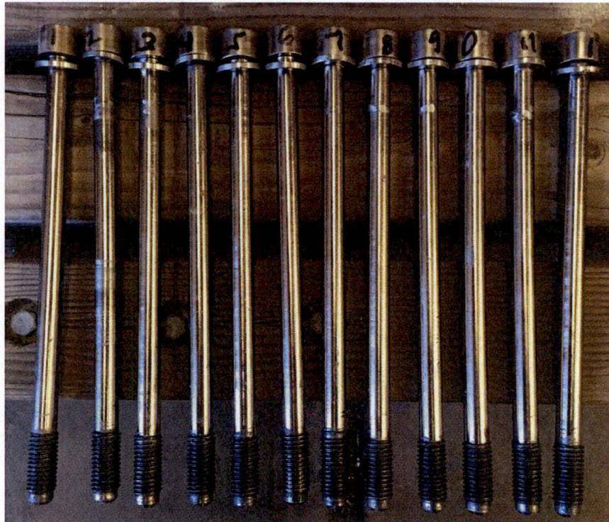
Figure 2.12.3-47 – Impact Limiter-3 Bolts after P3 and D3 Tests
