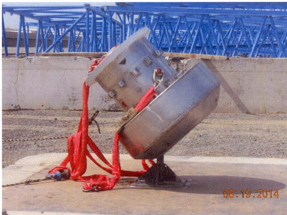
Figure 2.12.3-17 – CTU-1 Condition after P1 Puncture Drop Test
