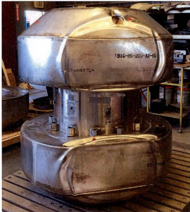
Figure 2.12.3-44 – CTU-3.4 Condition after D3 Free Drop Test
