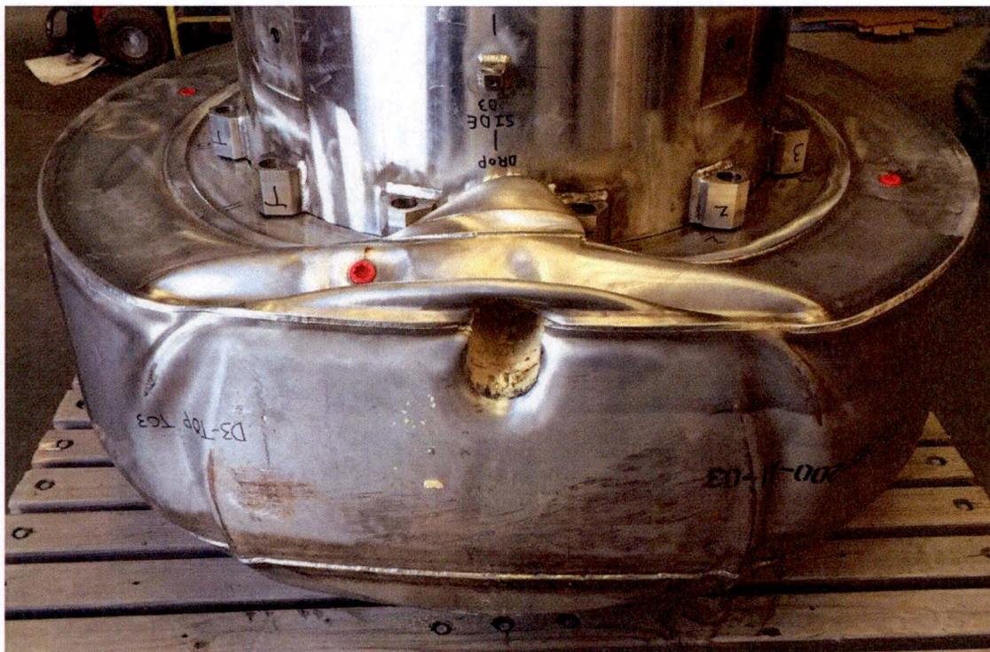
Figure 2.12.3-54 – Impact Limiter-4 Damage after D3 and P4 Tests
