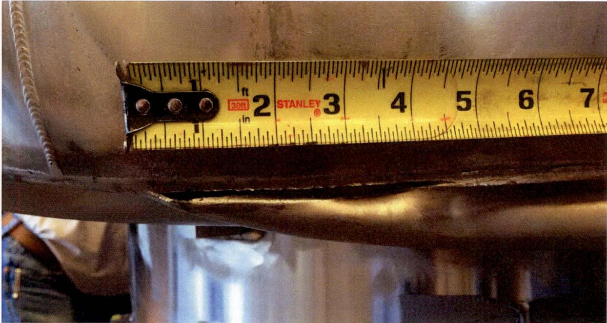
Figure 2.12.3-46 – Impact Limiter-3 Damage after P3 and D3 Tests
