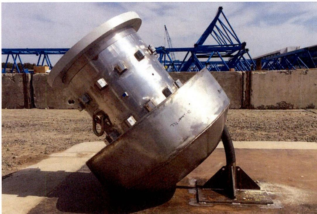
Figure 2.12.3-38 – CTU-3 Condition after P3 Puncture Drop Test
