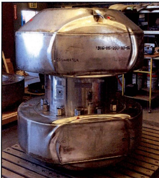
Figure 2.12.5-22 – CTU-3.4 Condition after D3 Free Drop Test
