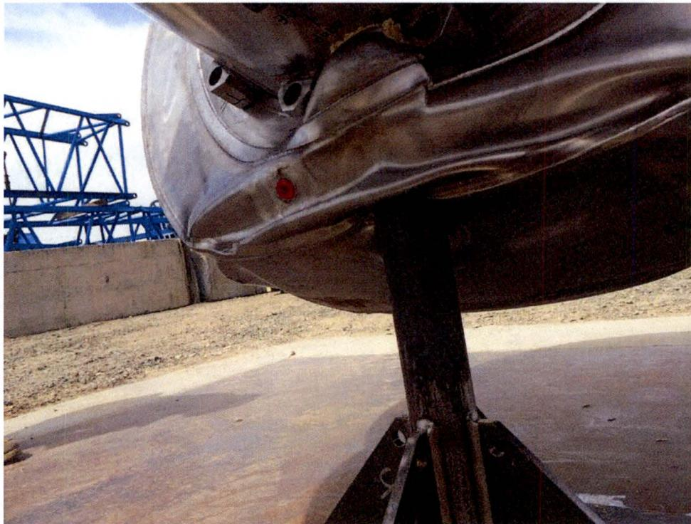
Figure 2.12.3-53 – CTU-4 Condition after P4 Puncture Drop Test
