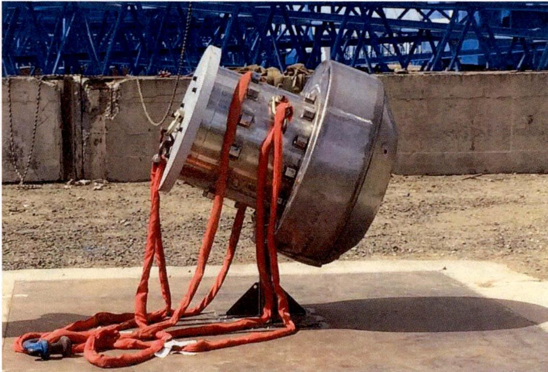
Figure 2.12.3-51 – CTU-4 Condition after P4 Puncture Drop Test
