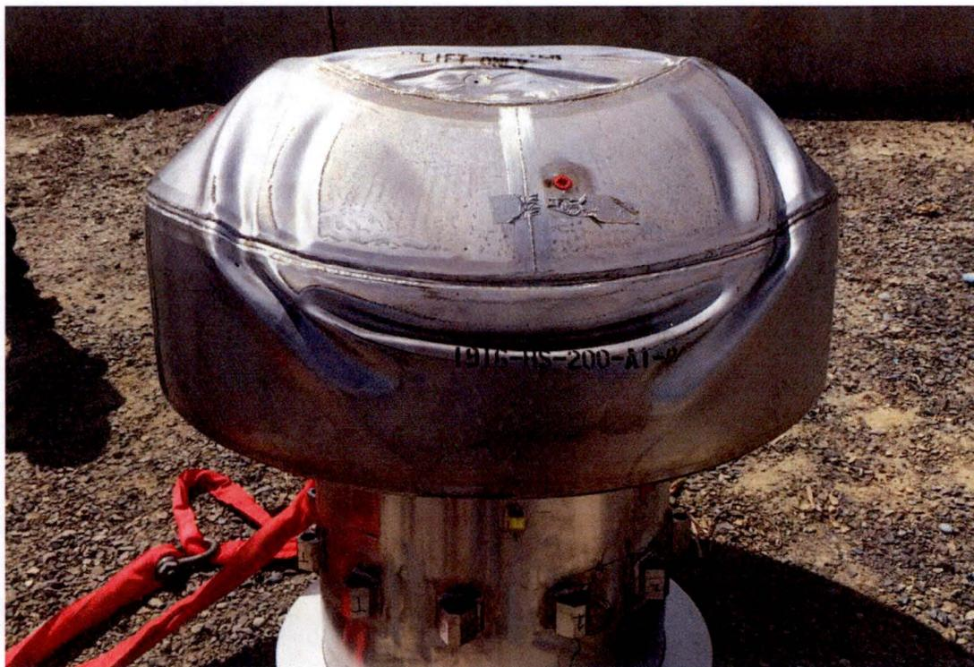
Figure 2.12.3-24 – CTU-2 Damage after D2 Free Drop Test
