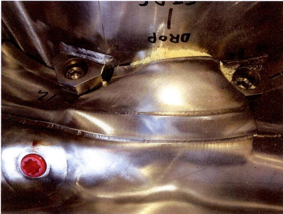
Figure 2.12.3-57 – Impact Limiter-4 Exit Damage after P4 Puncture Drop Test
