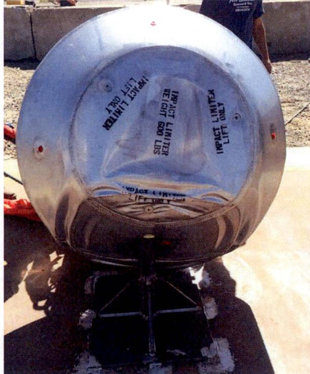
Figure 2.12.3-28 – CTU-2 Condition after P2 Puncture Drop Test
