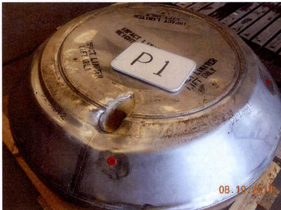
Figure 2.12.3-18 – Impact Limiter-1 Damage after P1 Puncture Drop Test
