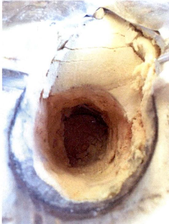
Figure 2.12.3-20 – Impact Limiter-1 Damage after P1 Puncture Drop Test
