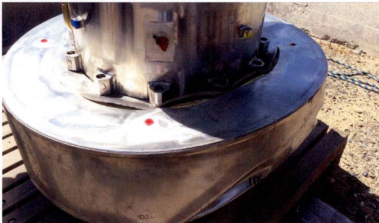
Figure 2.12.3-25 – CTU-2 Damage after D2 Free Drop Test
