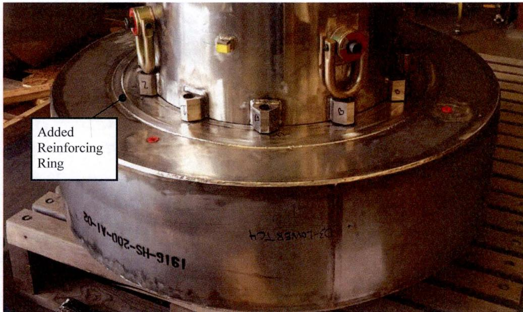
Figure 2.12.3-35 – Impact Limiter-3 with Reinforcing Ring
