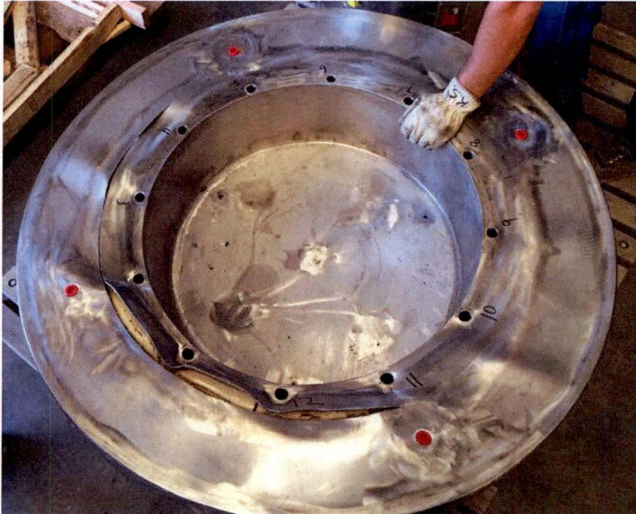
Figure 2.12.3-30 – Impact Limiter-2 Weld Failure after D2 and P2 Tests
