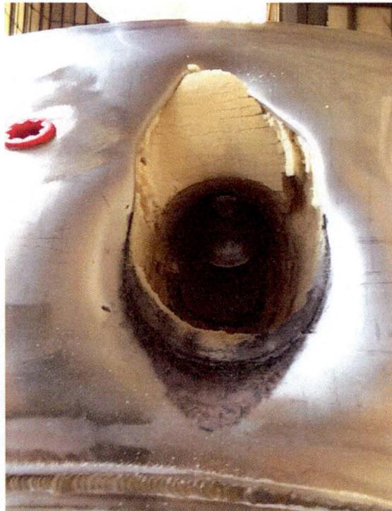
Figure 2.12.3-40 – Impact Limiter-3 Damage after P3 Puncture Drop Test
