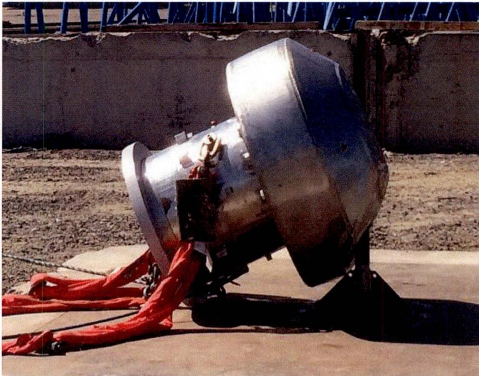
Figure 2.12.3-27 – CTU-2 Condition after P2 Puncture Drop Test
