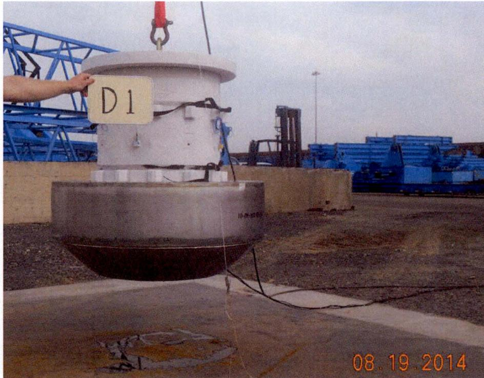
Figure 2.12.3-13 – CTU-1 Free Drop Test D1 Orientation
