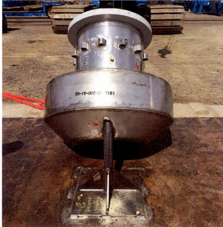
Figure 2.12.3-39 – CTU-3 Condition after P3 Puncture Drop Test
