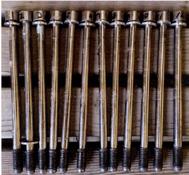
Figure 2.12.3-61 – Impact Limiter-4 Bolts after D3 and P4 Tests
