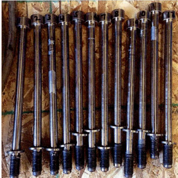
Figure 2.12.3-34 – Impact Limiter-2 Bolts after D2 and P2
