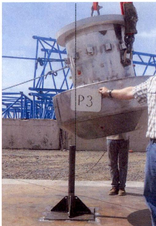
Figure 2.12.3-37 – CTU-3 Puncture Drop Test P3 Orientation
