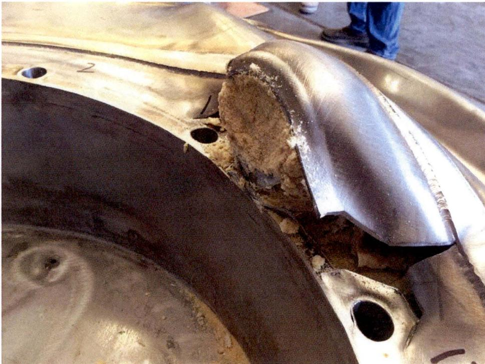
Figure 2.12.3-58 – Impact Limiter-4 Exit Damage without Cask
