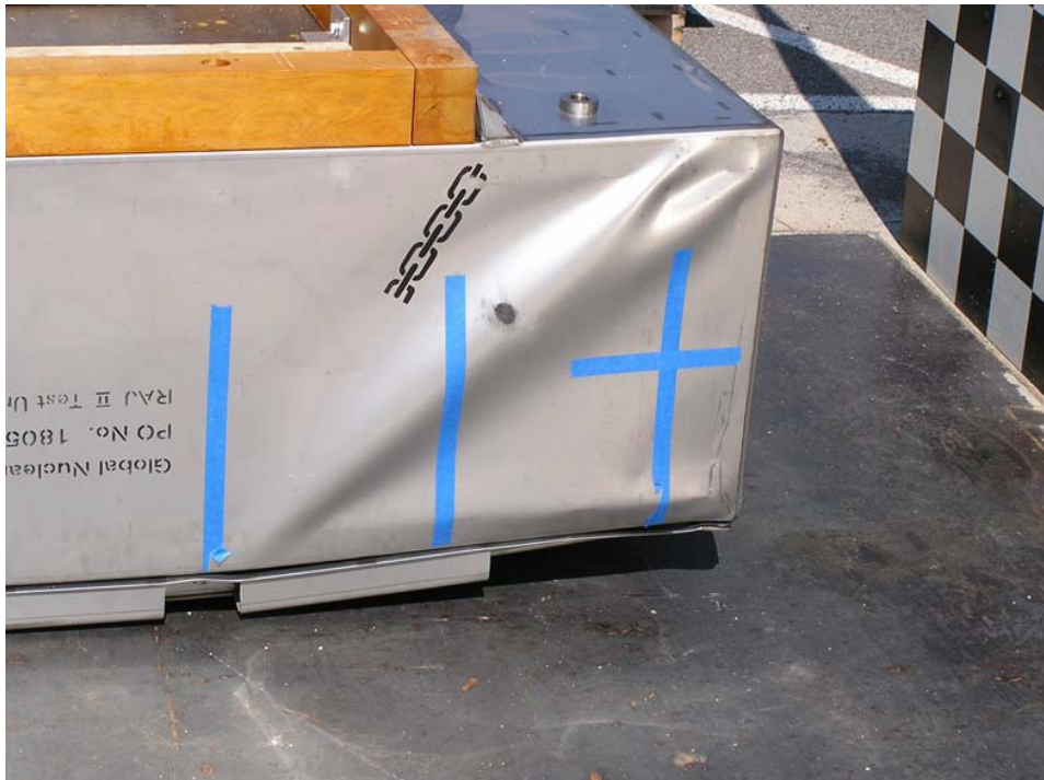
Figure 2-29 Primary Impact End Slap-down Damage
