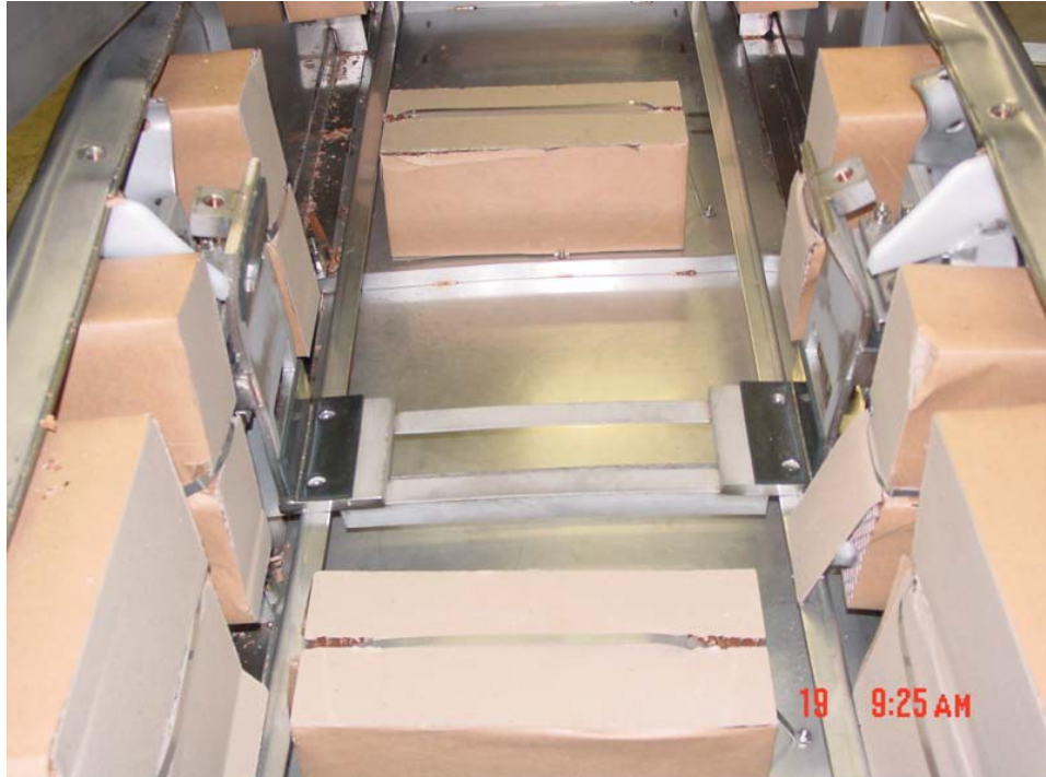
Figure 2-37 Internal Damage to Outer Container CTU 1
