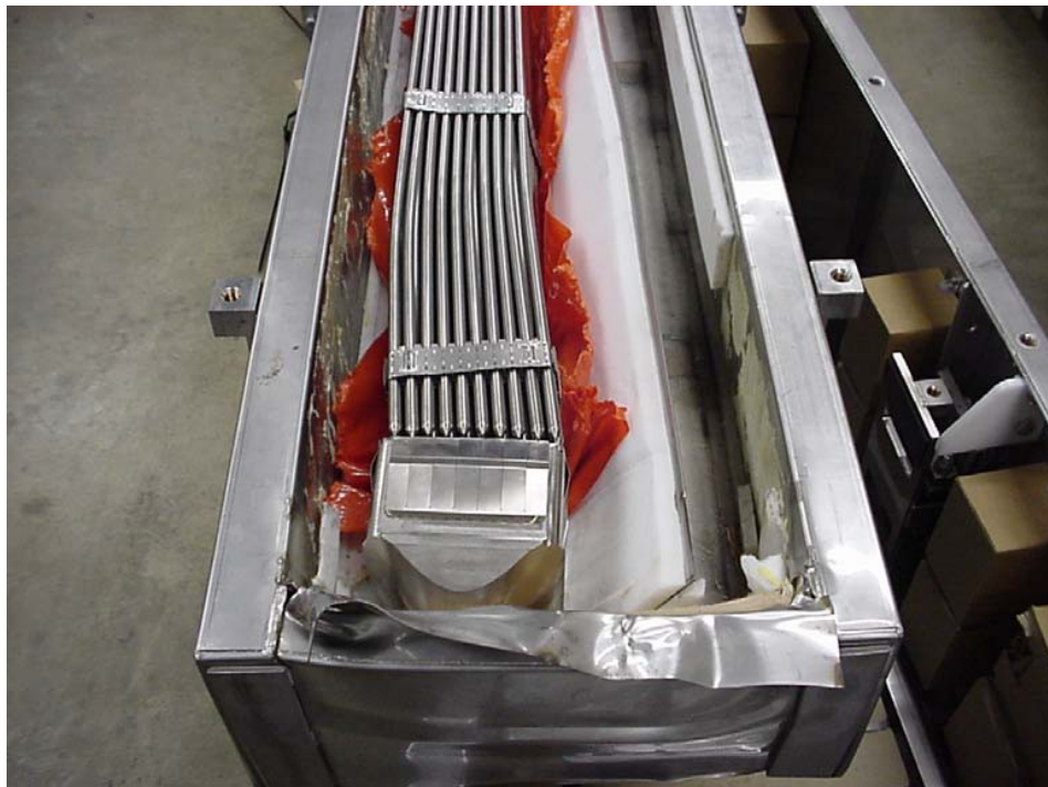
Figure 2-40 Internal Damage to CTU 2
