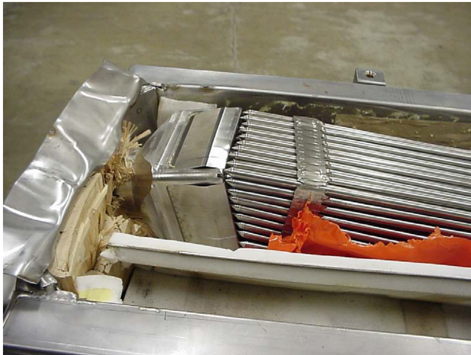
Figure 2-41 Fuel Damage CTU 2
