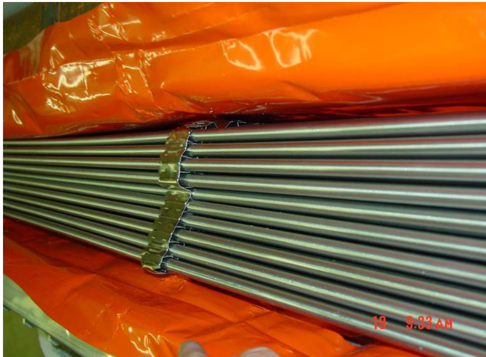
Figure 2-39 Damage to Fuel in CTU 1
