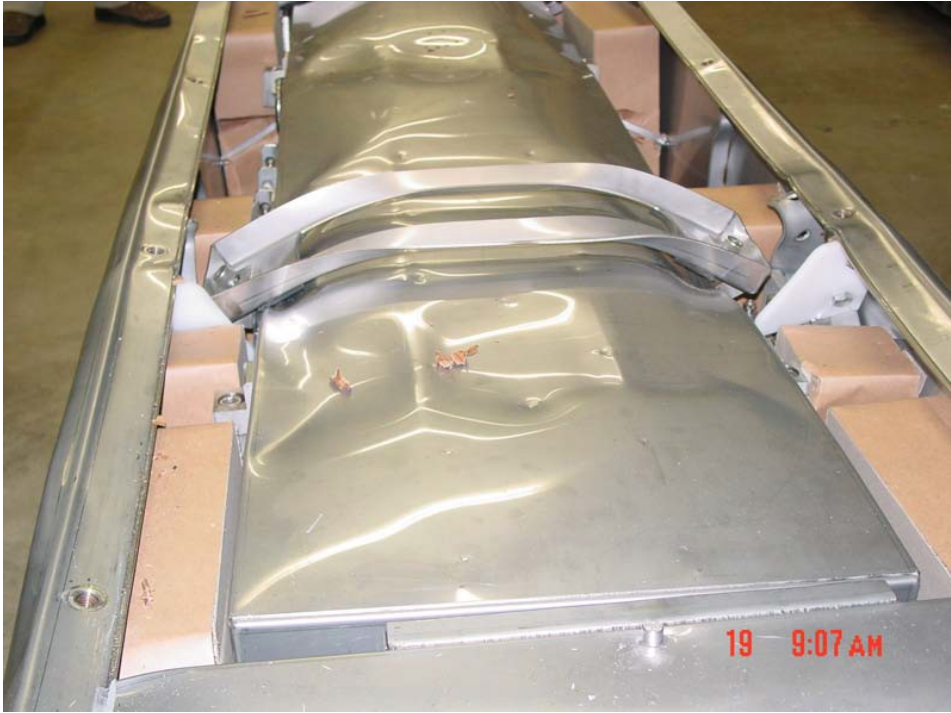
Figure 2-36 Damage Inside Outer Container to CTU 1
