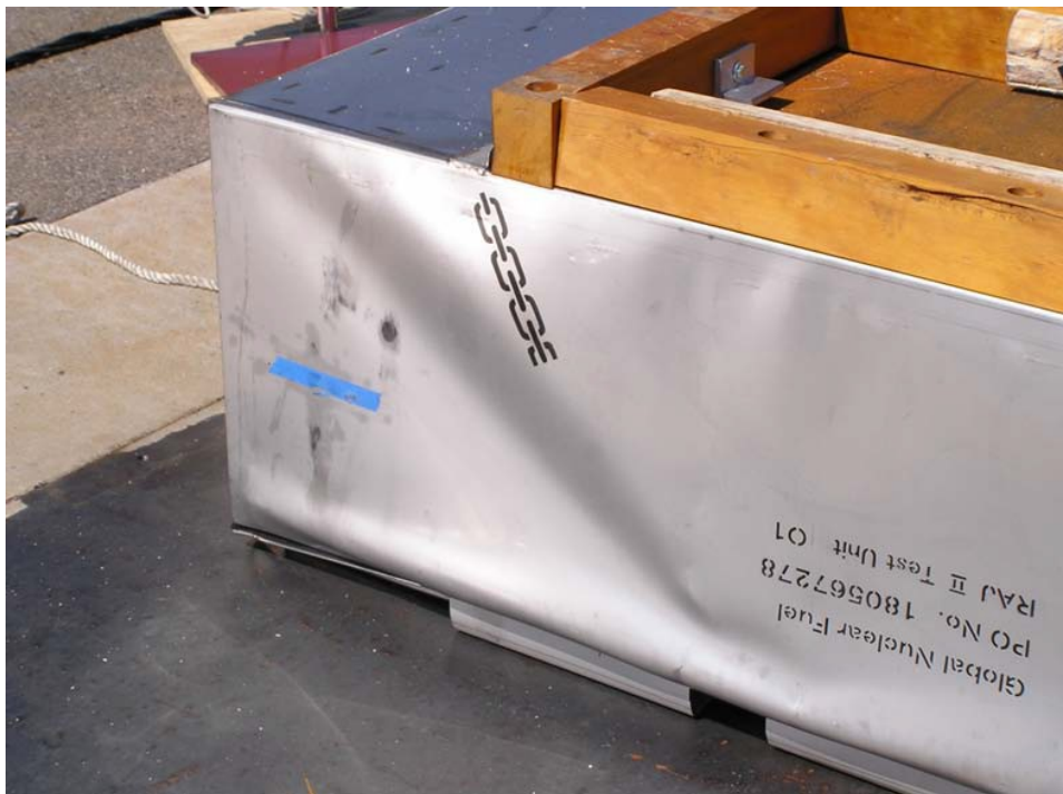
Figure 2-30 Secondary Impact End Damage
