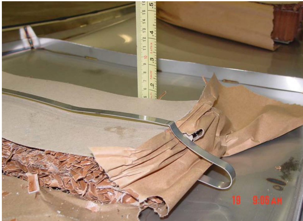
Figure 2-38 Lid Crush on CTU 1
