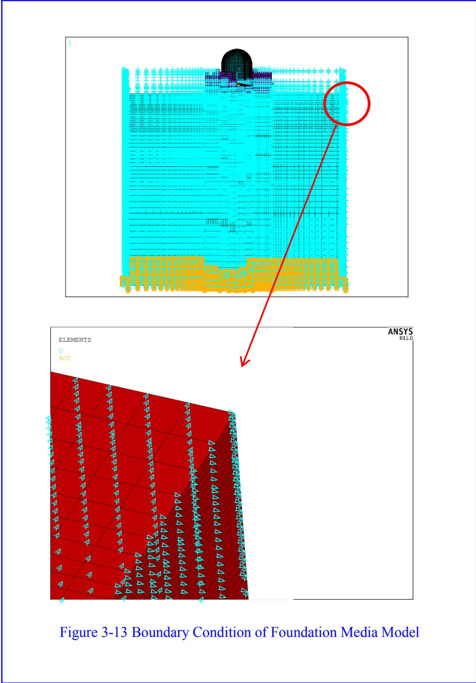
Figure 3-13 Boundary Condition of Foundation Media Model
