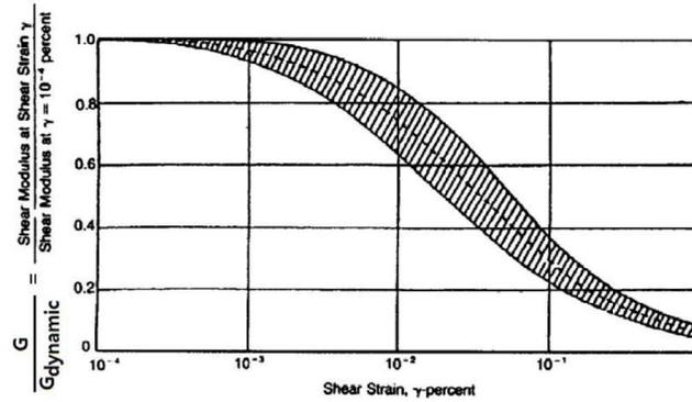
Figure 2-5 Variation of Shear Modulus with Shear Strain for Sands
