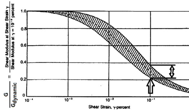
Figure 2-6  $G/G_{dynamic}$  of Soil at strain level 0.1%
