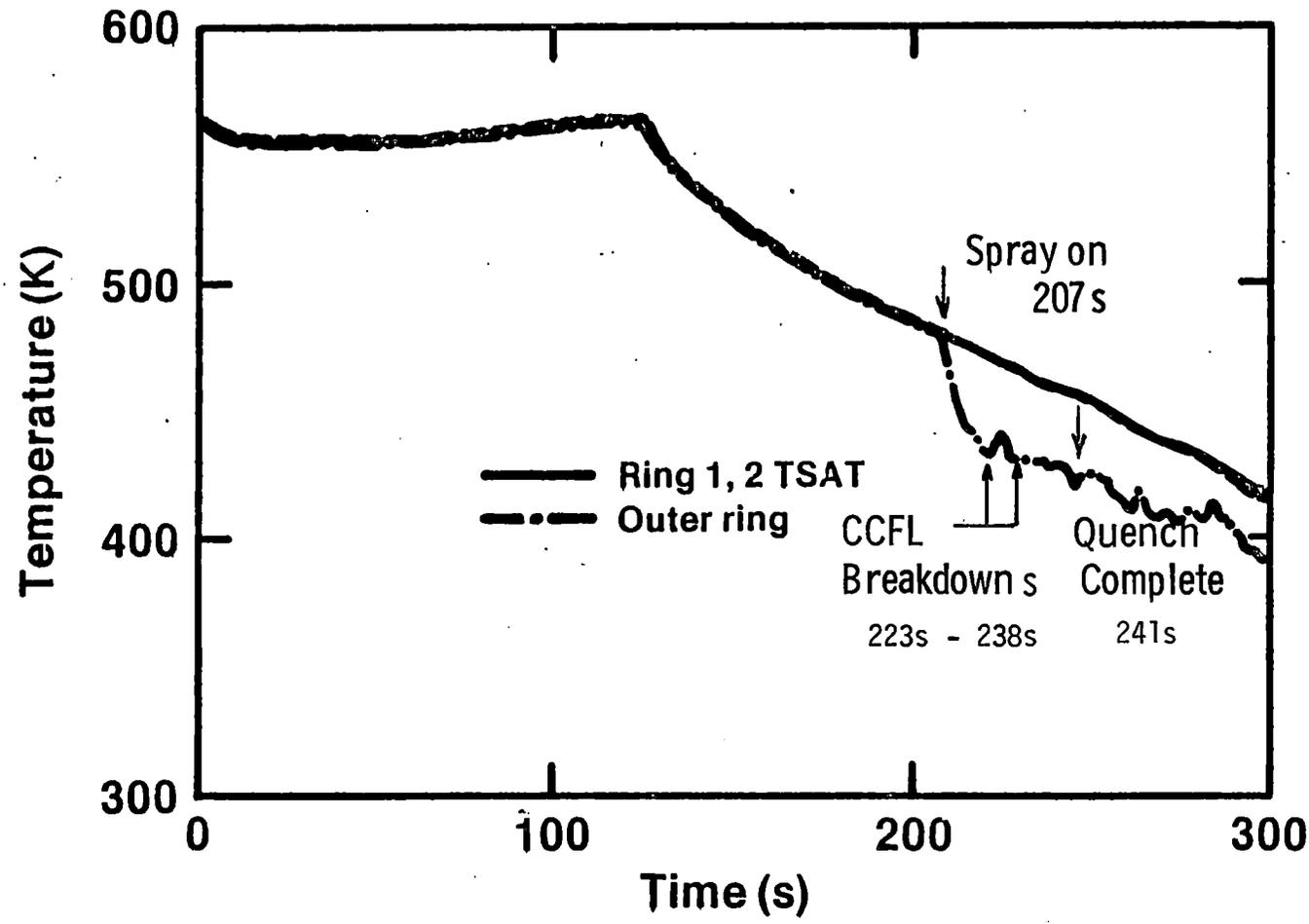
FIGURE A-3. SMALL BREAK CALCULATIONS
