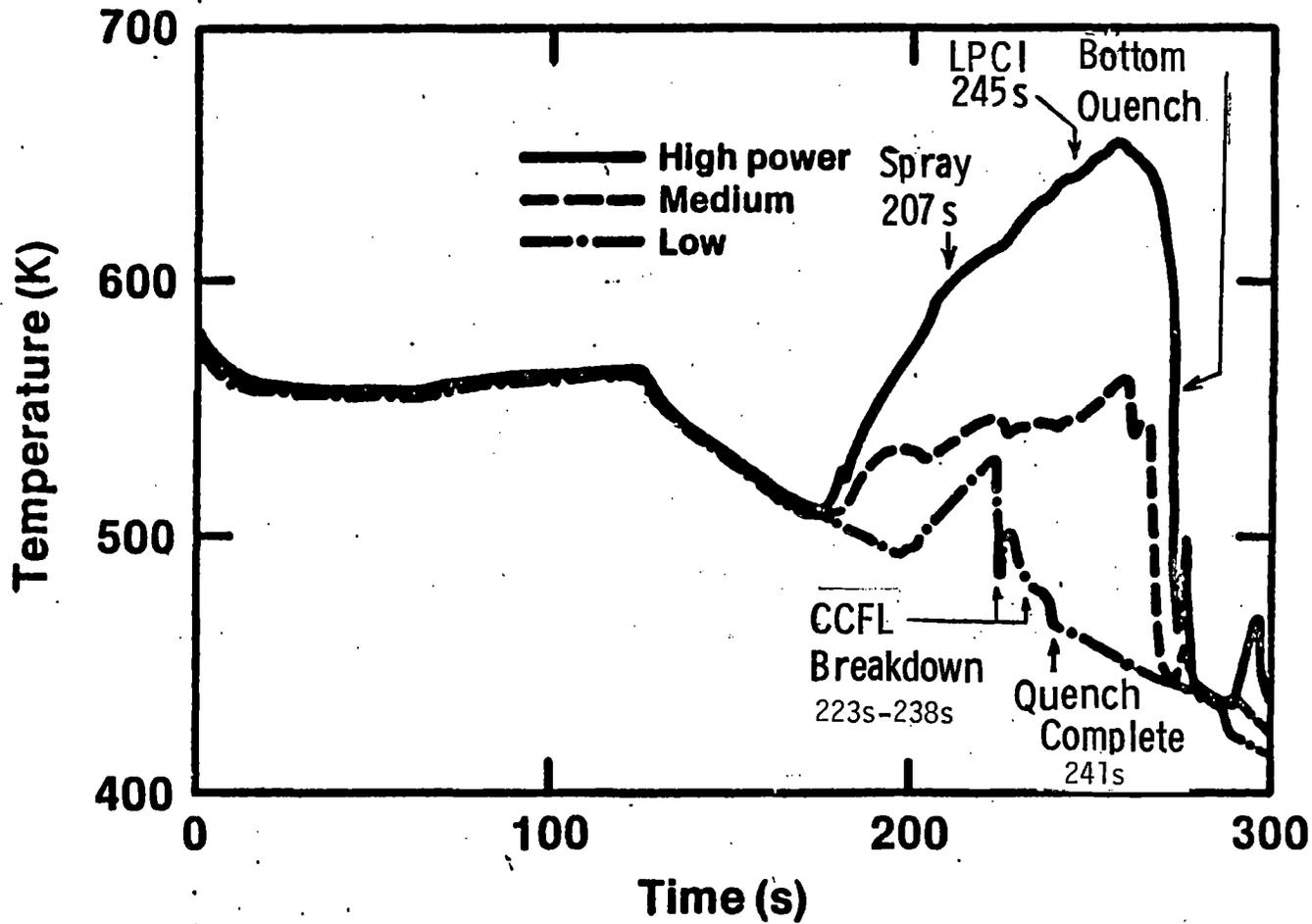
FIGURE A-4. SMALL BREAK CALCULATIONS
