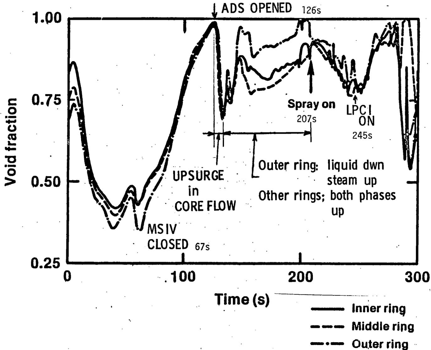
FIGURE A-2. SMALL BREAK CALCULATIONS
