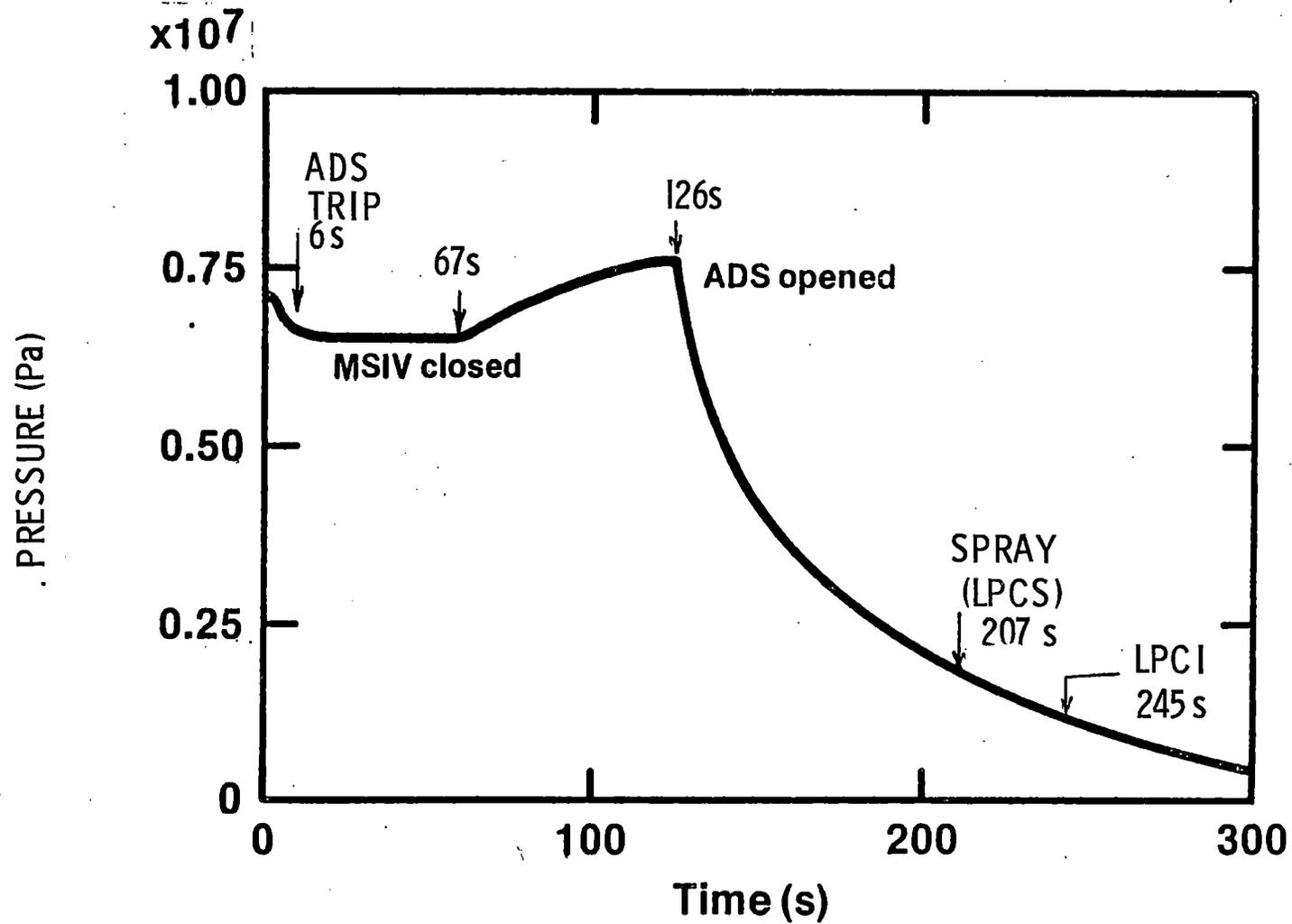
FIGURE A-1. SMALL BREAK CALCULATIONS
