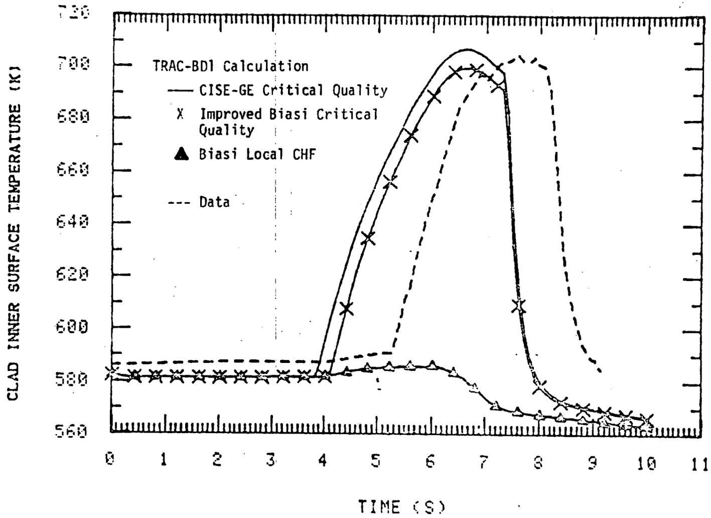
Figure 11. Comparison of TRAC-BD1 with GE Boiling Transition Data Obtained From Elevation 2 Rod Temperature Transient  $T_{CHF}$  Run 110.
