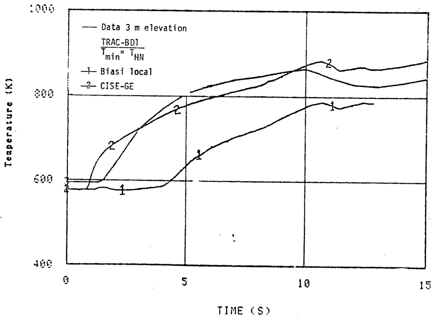
Figure 10. Data Obtained from TLTA Data, CISE-GE and Biasi Local.
